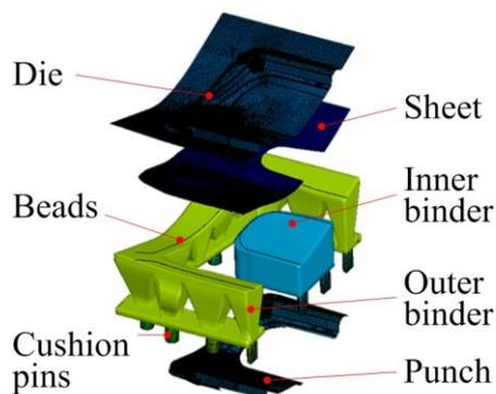
Figure 10; FE model with elastic BH [Altan et al., 2006]
