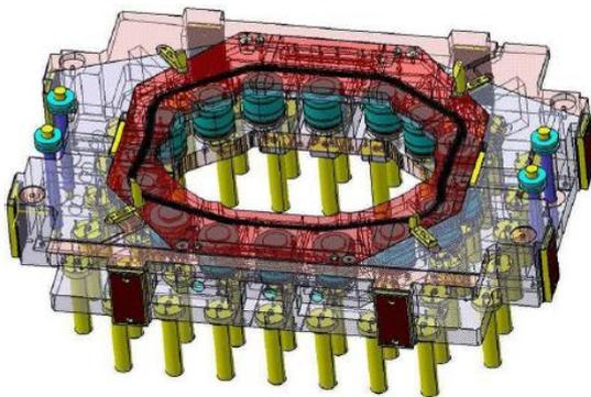
*Figure 6; In-die multi-point cushion system with Nitrogen Cylinders [Rittmeier, 2007]*
