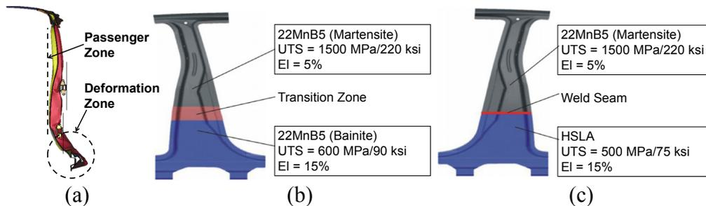
**Figure 3: (a) Side view of a B-pillar after crash [8]. (b) Tailored properties or (c) TWBs may improve elongation in the deformation zone [5].**
