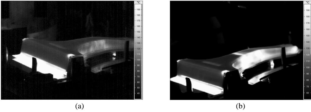
Figure 5: After-quench temperature for (a) constant thickness and, (b) variable thickness blank.
