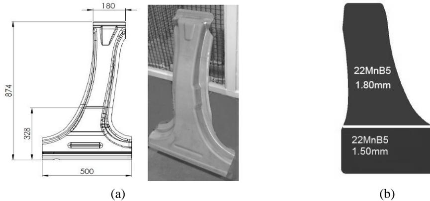
**Figure 2:** (a) B-pillar design (dimensions in mm) and product; (b) Sketch of the tailor-rolled blanks.
