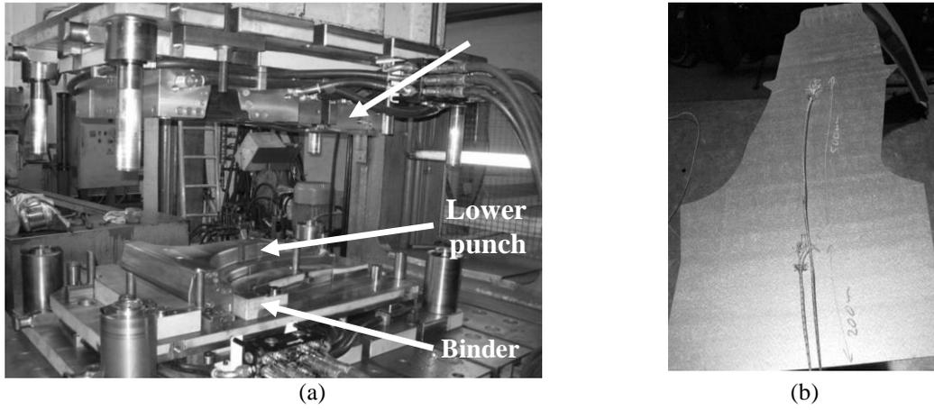
**Figure 3:** (a) Hot-stamping tools mounted on the hydraulic press, (b) Thermocouples installed in the blank.
