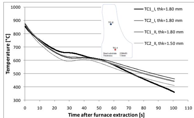
**Figure 4:** Temperature evolution for one sample, of each studied case, air-cooled after austenization.
