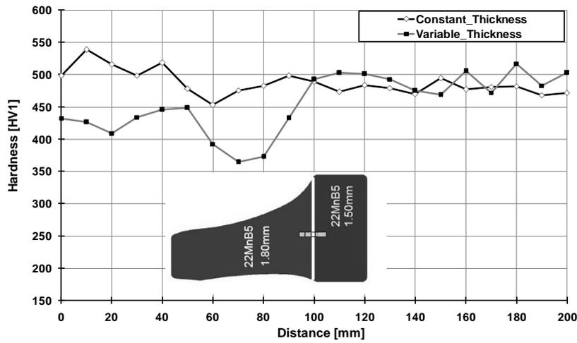
Figure 6: Vickers hardness taken at the transition zone of the two studied variants.
