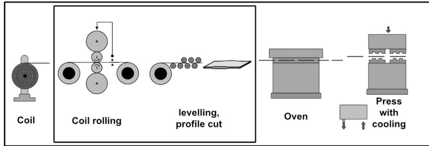
Figure 1: Hot stamping process of tailor rolled blanks [1].
