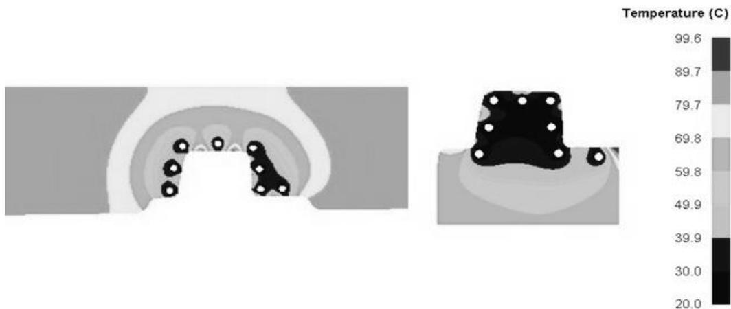
**Figure 5:** Temperature distribution in the die (left) and punch (right) at the end of 10 forming cycles
