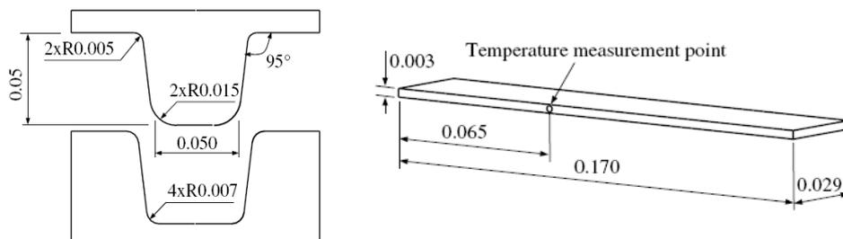
Figure 1: Die geometry for hat shape, All dimensions are in m [8]
