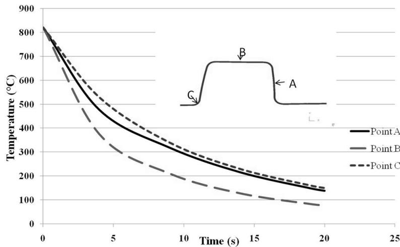
**Figure 6:** Variation of temperature at points A, B and C during quenching (20 s)
