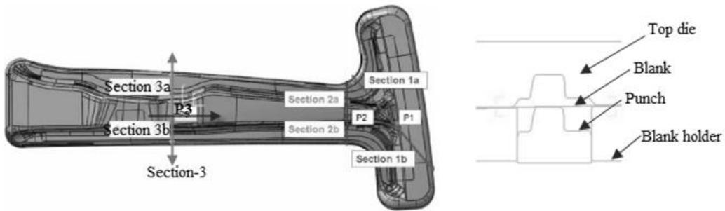
Figure 3: Section-3 as given in [7] and initial forming simulation setup for section-3
