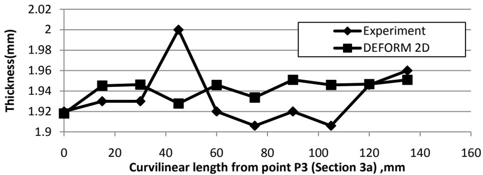
Figure 4: Comparison of thickness distribution from experiment and simulation for section- 3a
