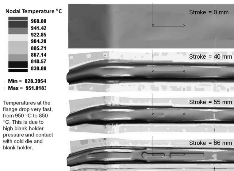
**Figure 8:** Preliminary forming simulation of a part geometry (Case 2) using PAMSTAMP™
