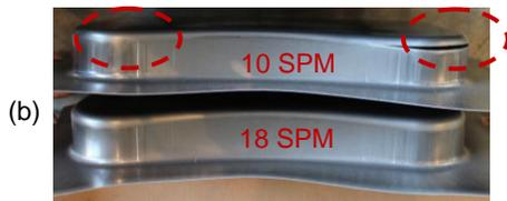
Figure 9: Results of deep drawing tests with dry film lubricant under different crank motion based forming speeds, stroke 60.8 mm: (a) 10 SPM, crack at right corner and necking at left corner, (b) 18 SPM, defect free formed part
