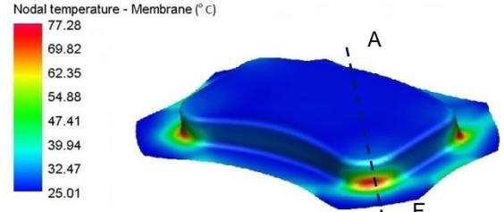
Figure 15: Temperature distribution in the drawn part at forming speed 310 mm/s, stroke = 60 mm
