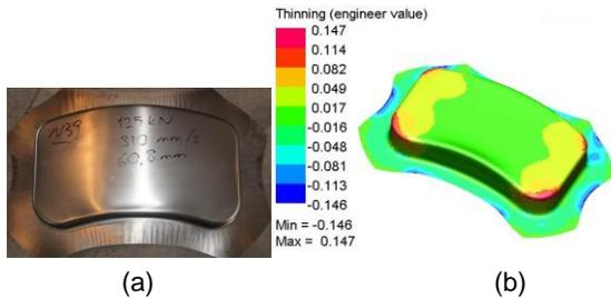
Figure 6: (a) Defect free formed part (draw depth 60.8 mm); (b) thinning distribution of simulated part in PAMSTAMP.
