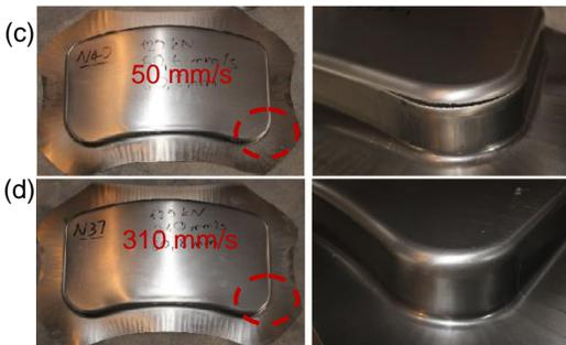
Figure 10: Results of deep drawing tests with dry film lubricant under different constant forming speeds, stroke 60.8 mm: (c) 50 mm/s, crack at right corner, (d) 310 mm/s, defect free formed part
