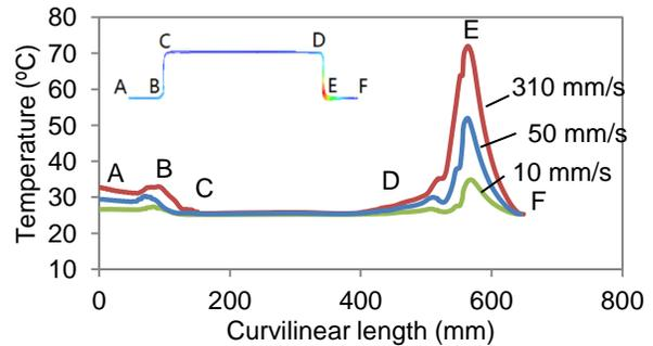
Figure 16: Predicted temperature distributions in the drawn part along the selected section A-F at different forming speeds, stroke = 60 mm
