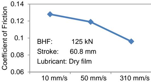
Figure 14: Predicted coefficient of friction at different forming speeds
