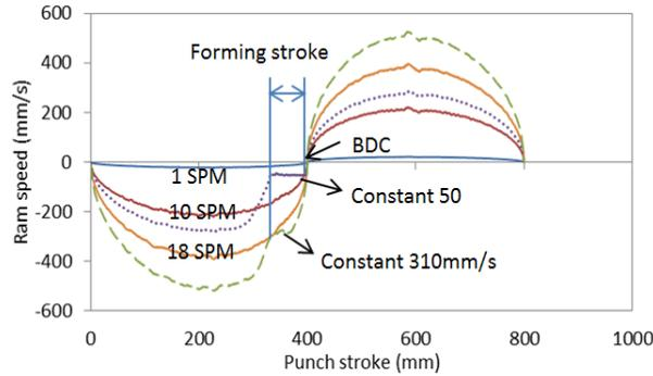
Figure 4: Ram speed profiles with crank motion (1 SPM, 10 SPM and 18 SPM) and constant (50 mm/s and 310 mm/s) during deformation.
