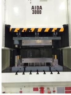
Figure 3: Experimental deep drawing tooling assembled in the 300 ton servo press
