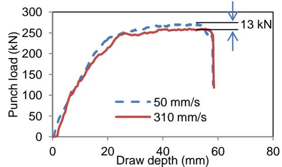
Figure 12: Load-stroke curves at forming speeds 50mm/s and 310mm/s, with dry film lubricant (BHF 125 kN, stroke 60.8 mm)
