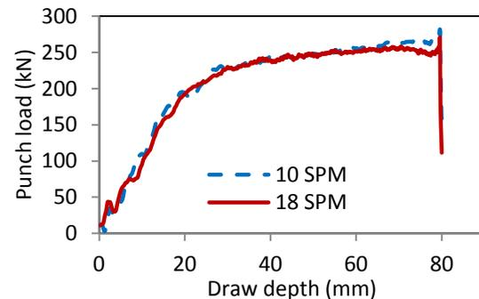
Figure 13: Load-stroke curves at forming speeds 10 SPM and 18 SPM, with oil lubricant (BHF 125 kN, stroke 80 mm)
