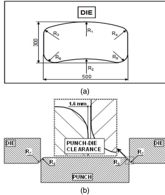
Figure 2: (a) Top and (b) cross-sectional view of deep drawing tooling, dimensions are in mm ( $R_1=1501.6$ ,  $R_2=1998.4$ ,  $R_3=51.6$ ,  $R_4=55.6$ ,  $R_5=61.6$ ,  $R_6=66.6$ ,  $R_7=20$ ,  $R_8=10$ ).
