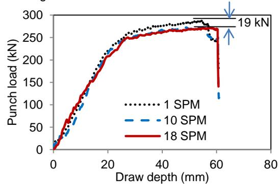
Figure 11: Load-stroke curves at forming speeds 1 SPM, 10 SPM and 18 SPM, with dry film lubricant (BHF 125 kN, stroke 60.8 mm)
