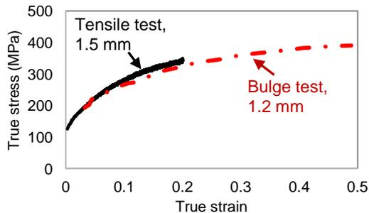
Figure 1: Flow stress curves of Al 5182-O obtained from tensile test and VPB test.
