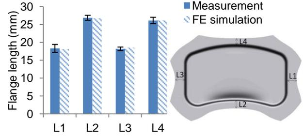
Figure 7: Comparison of flange lengths between experiment and FE simulation (COF 0.1 was applied).
