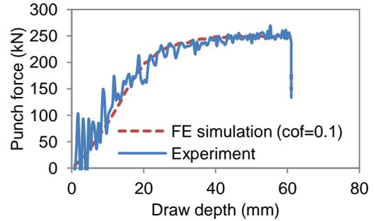
Figure 8: Load-stroke curves from experiment and FE simulation (COF 0.1 was applied).
