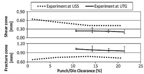
Fig. 5. Sheared edge geometries from blanking experiments at USS and UTG.
