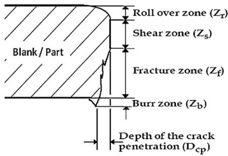
Fig. 1. Geometric parameters of the blanked edge.
