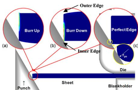
Fig. 4. Schematic of hole flanging simulation with burr orientation (a) up and (b) down and (c) perfect edge using a conical punch.
