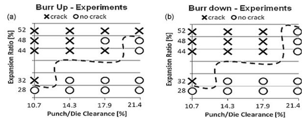
Fig. 3. Expansion ratios in form of an evaluation matrix for two cases (a) burr up and (b) burr down (from the experiments at UTG).
