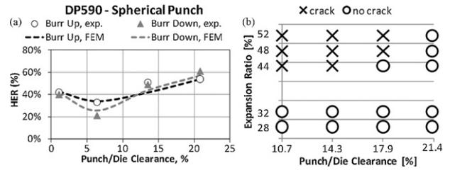
Fig. 9. (a) Comparison of HER (at fracture) for a spherical punch, from FE simulations with Eq. (4) and experiments at USS, and (b) prediction of edge cracking occurrence in hole expansion tests at UTG (burr down).
