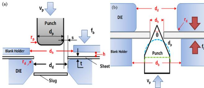
Fig. 2. Schematics of (a) blanking and (b) hole expansion (flanging).
