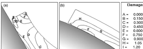
Fig. 8. Distributions of DV in hole expansion for (a) conical and (b) spherical punch, (orig. blanked hole radius = 5 mm, flanged inner hole radius = 7.5 mm).
