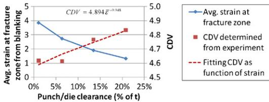
Fig. 7. Average effective strain at the fracture zone obtained from blanking simulation at different punch/die clearances, and CDV obtained from FE simulation of hole expansion for USS tests (conical punch).
