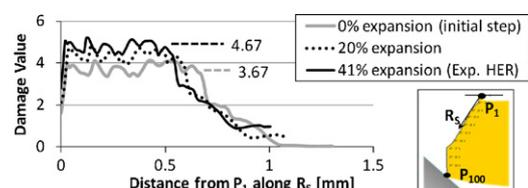
Fig. 6. Distribution of damage value over the sheared edge for burr up at different expansion ratios (punch/die clearance = 1.1%).
