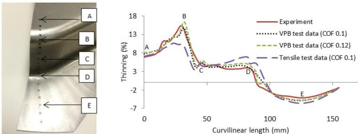
Figure 6: Comparison of measured and predicted thinning at the critical corner of the drawn part (Material: Al 5182-0, thickness = 1.2 mm, BHF = 150 ton, COF = 0.1 and 0.12, Draw Depth = 75 mm, Ram speed = 310 to 0 mm/s)
