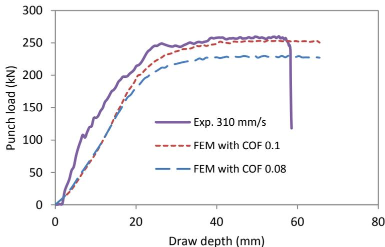
Figure 8: Comparison of the load versus stroke curve measured from experiment (solid line) and FE prediction with two different COF, in forming Al 5182-0.
