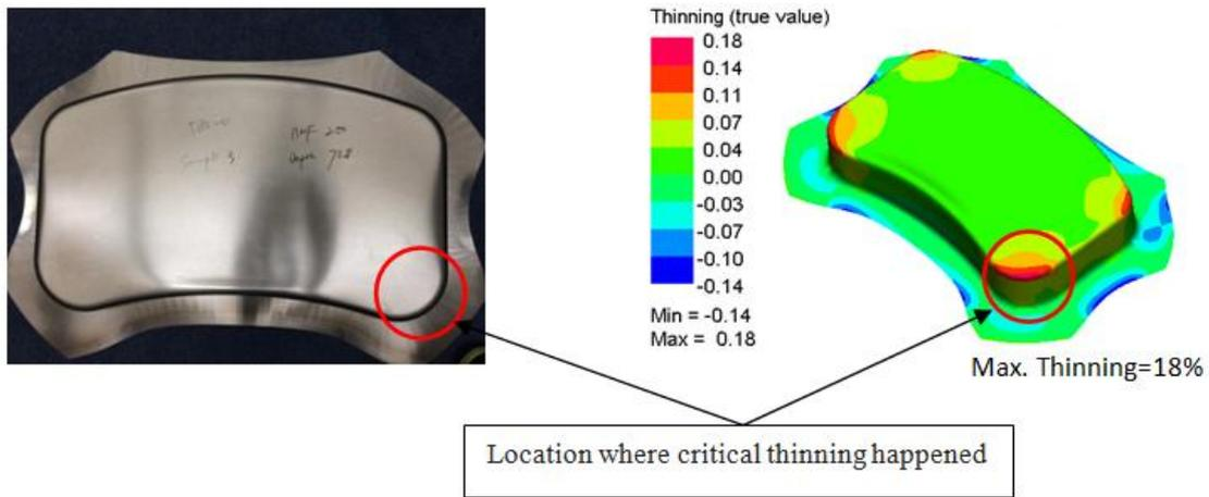
Figure 5: Aluminum panel formed by 300 Ton servo drive press and simulation results of the same operation
