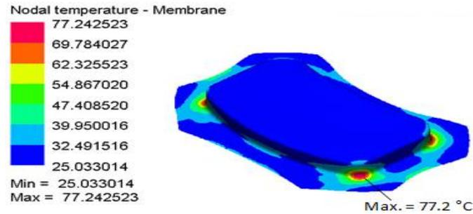
Figure 7: Temperature predictions during drawing of Al 5182-O (PAMSTAMP). Maximum temperature at the part corner is about 80°C.
