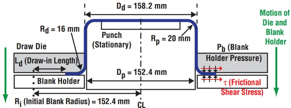
Figure 3: The schematic of the Cup Draw Test (CDT) to evaluate stamping lubricants [5]
