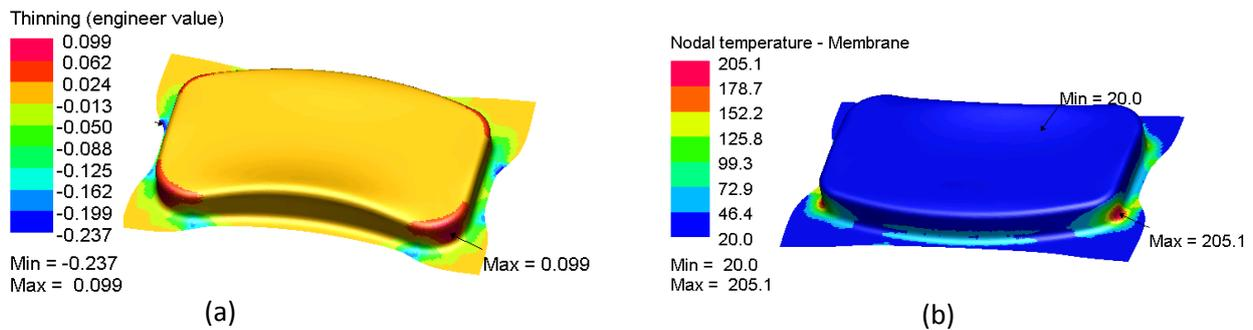
Figure 9: (a) Thinning and (b) Temperature predictions for 55mm deep drawn DP980 sheet with 1.2mm thickness (PAMSTAMP)
