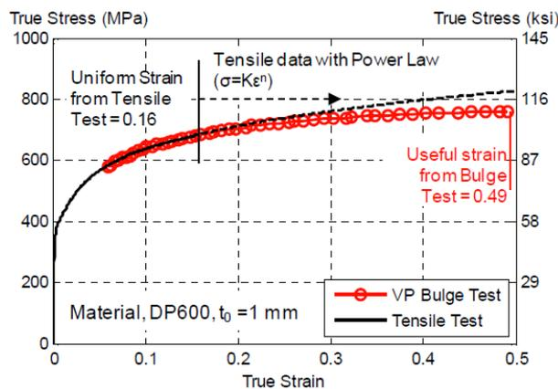
Figure 2: Comparison of flow stress determined by tensile test and bulge test for DP 600 steel [4].
