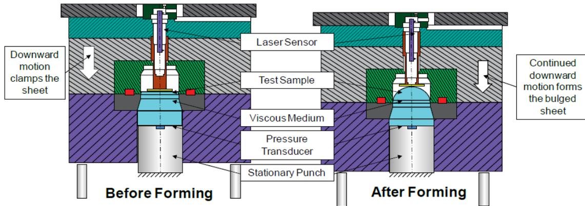
Figure 1: Viscous pressure Bulge Test. The flow stress is determined by inverse FE analysis using pressure and dome height measured during the test [4].
