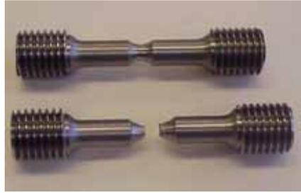
Fig. 15 Notched tensile test specimen before-and- after fracture /11/.
