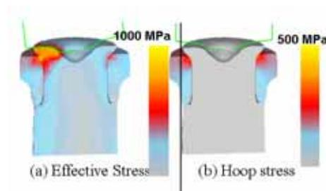
Fig. 10 Residual stresses predicted by FE simulation in the spindle bearing assembly at the end of orbital forming /6/.
