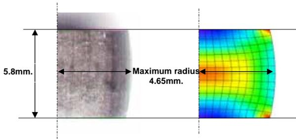
Fig. 4 Comparison of deformed shape in the compression test from FE simulation and experiment for the optimized material parameters ( $\sigma = 795.7\epsilon^{0.15} MPa$ ) and friction conditions (friction factor  $m = 0.15$ ) /3/.
