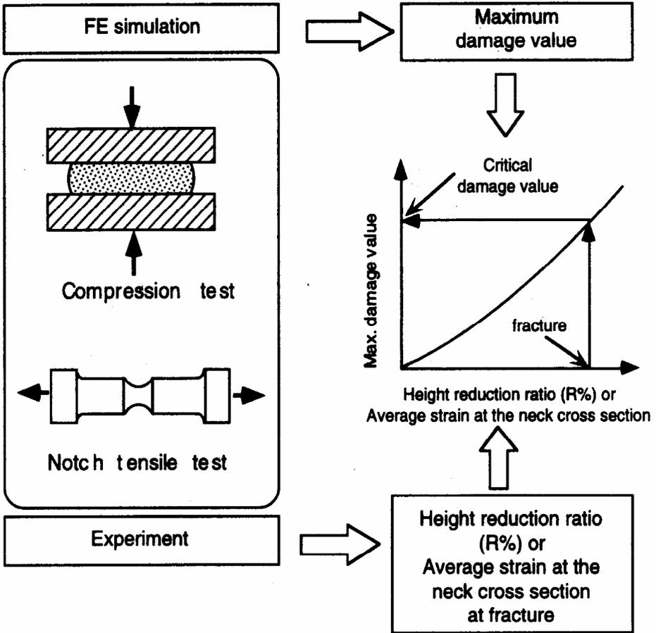
Fig. 12 Proposed approach to obtain critical damage value from compression and notch tensile test in conjunction with FE simulations /9/.
