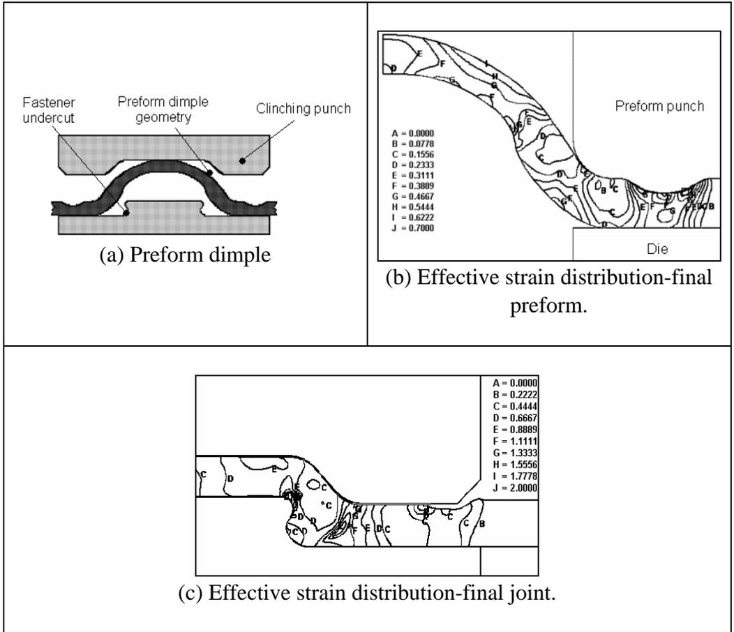
Fig. 8 FE simulation of clinching /5/.
