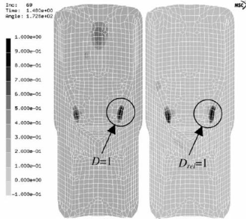
Fig. 23 Absolute and relative damage distribution of the MES in the fourth stage with original tools at  $173^\circ$  crank angle /14/.
