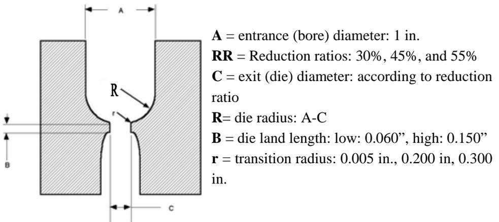
Fig. 16 Schematic representation of the parameters to be investigated during forward extrusion with spherical die.
