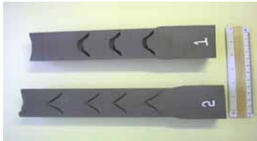
Fig. 2 Illustration of different chevron configurations /1/.
