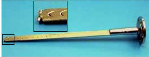
Fig. 1 Automotive axle shaft with chevrons /1/.
