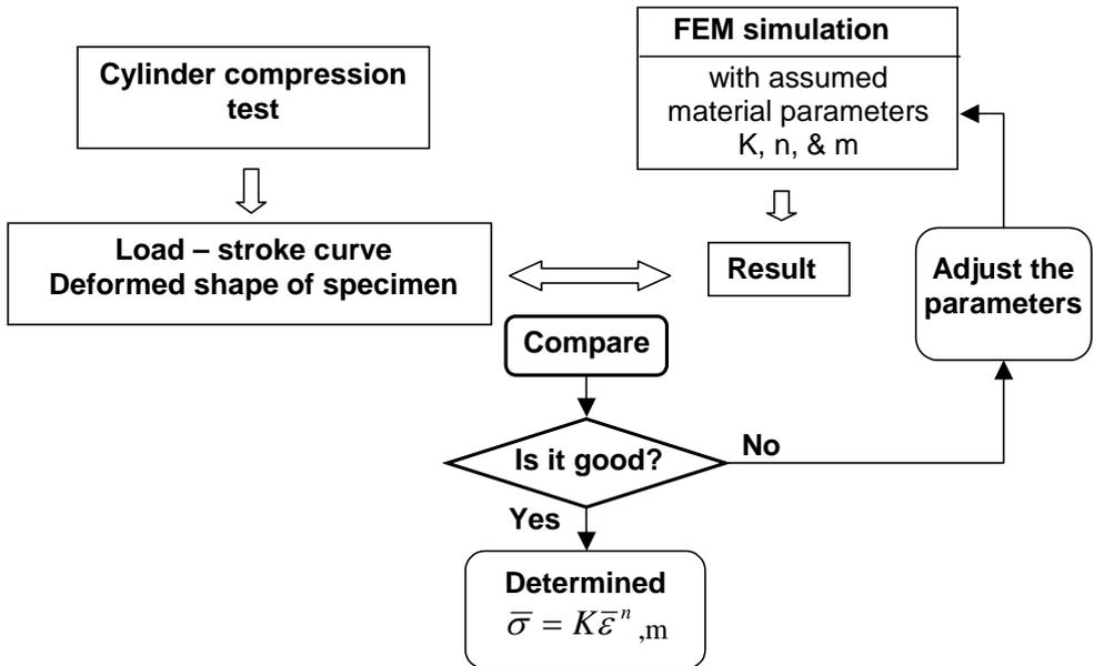
Fig. 3 Flow chart of the inverse analysis methodology to estimate flow stress using FE simulation /3/.
