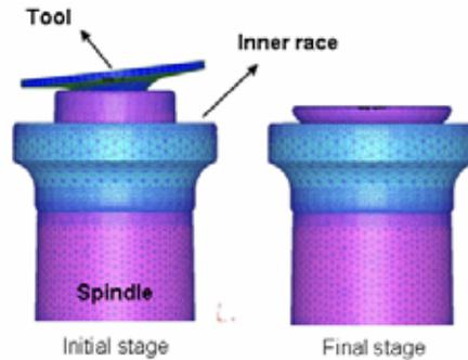
Fig. 9 FE model for orbital forming of spindle bearing assembly /6/.
