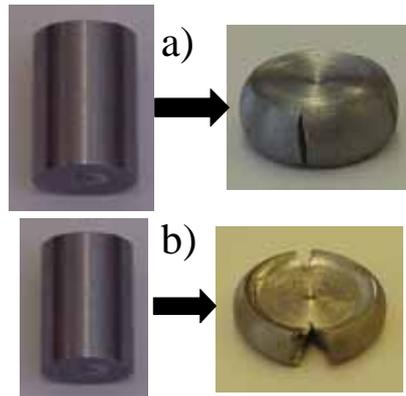
Fig. 14 Specimens for non-uniform compression test, a) SAE 1137 hot rolled, b) SAE 1524 spheroidized annealed /12/.
