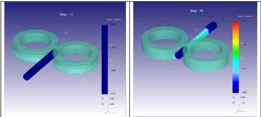
Fig. 11 Three dimensional FE simulation of reducer rolling.
