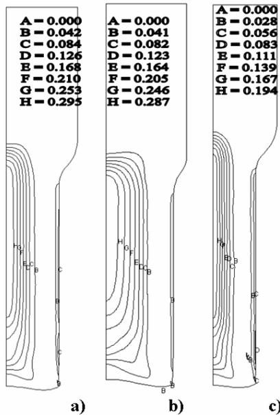
Fig. 19 Distribution of the damage value during several reductions in area: (a) 30%, (b) 45% and (c) 55% (B = 0.150” and r = 0.200”) /13/.
