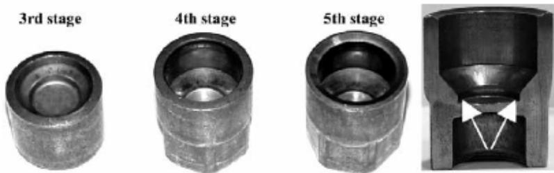
Fig. 22 Production sequence of the double cup and observed damage locations in the fourth stage /14/.
