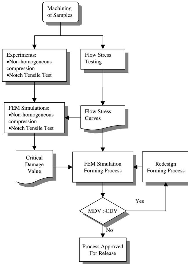
Fig. 13 Methodology to predict and prevent the formation of cracks /9/.
