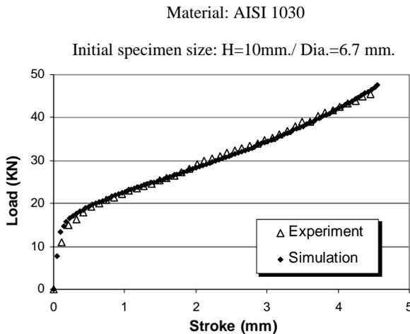
Fig. 5 Comparison of load stroke curve from FE simulation and experiment for the optimized material parameters ( $\sigma = 795.7\epsilon^{0.15} MPa$ ) and friction conditions (friction factor  $m = 0.15$ ) /3/.
