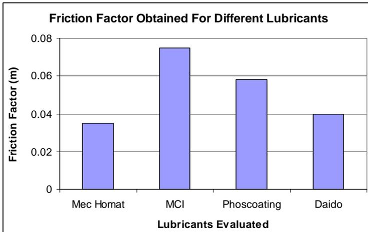
Fig.7 Ranking of the lubricants based on the friction factors obtained /4/.
