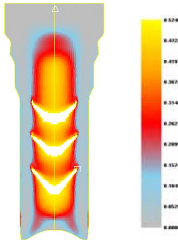
Fig. 20 Formation of chevron cracks during the third stage of three-pass forward extrusion using first pass as spherical die with material SAE 1137 (hot rolled) and its correspondent damage value distribution /12/.
