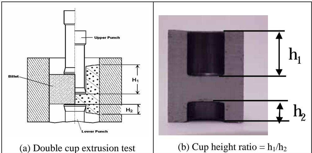
Fig. 6 Double cup extrusion test /4/.
