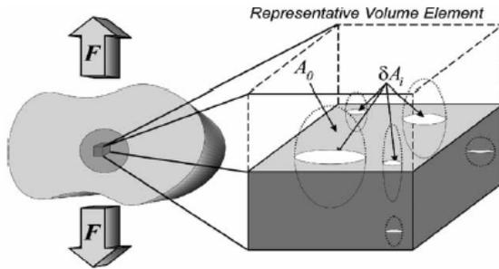
Fig. 21 Definition of Representative Volume Elements (RVE) and absolute damage ( $F$ =load acting on the body,  $A_0$  is the load carrying area,  $\delta A_i$  is the total cavity area) /13/.
