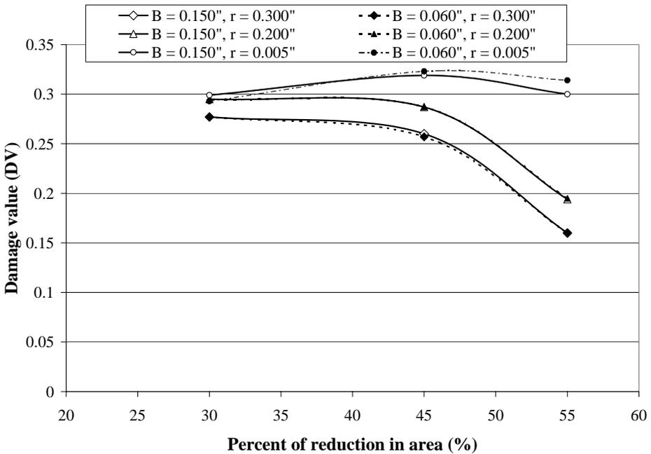
Fig. 17 Effect of reduction ratio on damage value in single-pass forward extrusion /12/.
