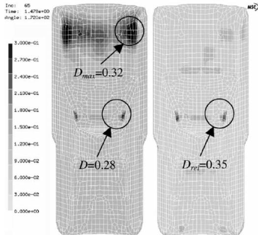
Fig. 24 Absolute and relative damage distribution of the MES in the fourth stage with modified tools at  $172^\circ$  crank angle /14/.
