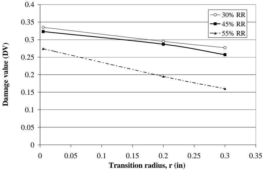
Fig. 18 Effect of transition radius for several reduction ratios (RR) /12/.
