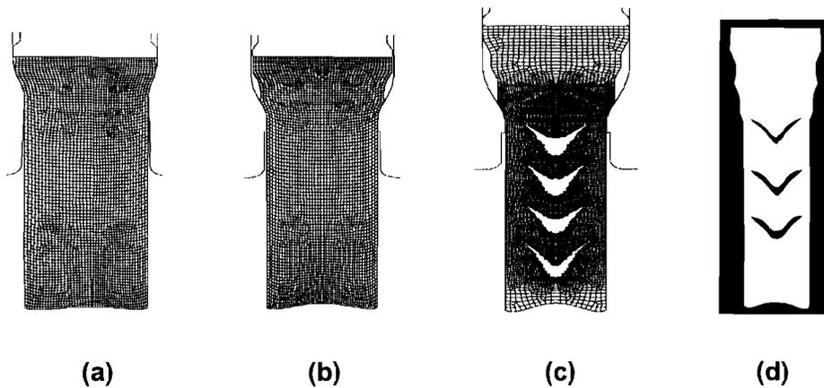
**Figure 5. Simulation of a) first, b) second, and c) third pass forward extrusion. The actual product (d) is also shown**
