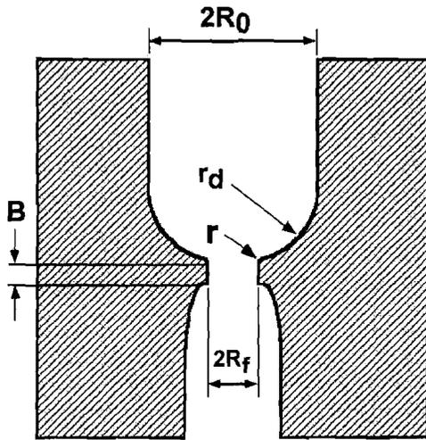
**Figure 9. Schematic representation of the parameters to be investigated during forward extrusion with spherical die.**
