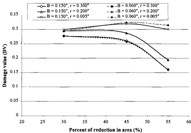
Figure 10. Effect of reduction ratio on damage value in single-pass forward extrusion
