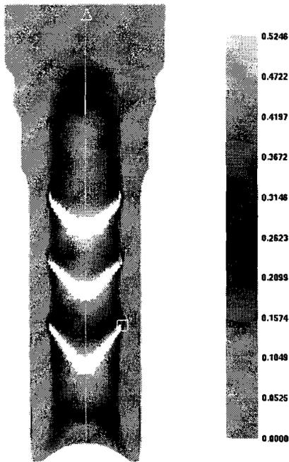
Figure 13. Formation of chevron cracks during three-pass forward extrusion using first pass as spherical die with material SAE 1137 (hot rolled) and its correspondent
