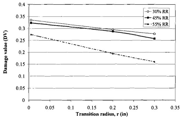
Figure 11. Effect of transition radius on Damage value for several reduction ratios
