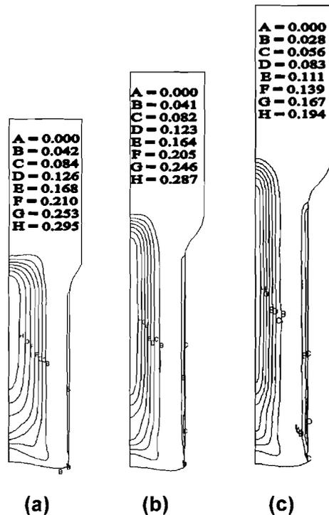
Figure 12. Distribution of the damage value during several reductions in area: (a) 30%, (b) 45% and (c) 55% (B=0.150" and R = .200").
