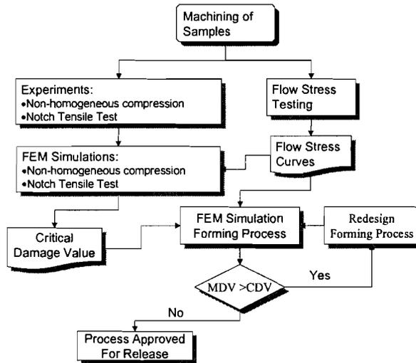
**Figure 4. Methodology to predict & prevent the formation of cracks in metal forming operations**
