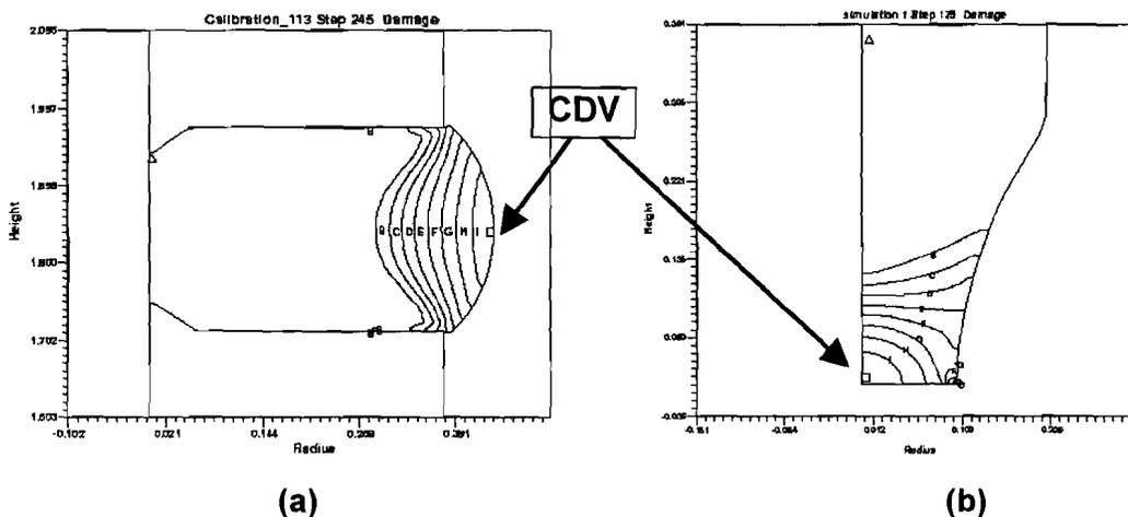
**Figure 8. Distribution of the critical damage value for material SAE 1137 (hot rolled) a) non-homogeneous compression and b) notched tensile test.**
