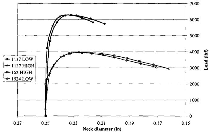
**Figure 7. Neck diameter-load curve for tensile tests with notched specimens of SAE 1137 hot rolled and SAE 1524 spheroidized annealed.**
