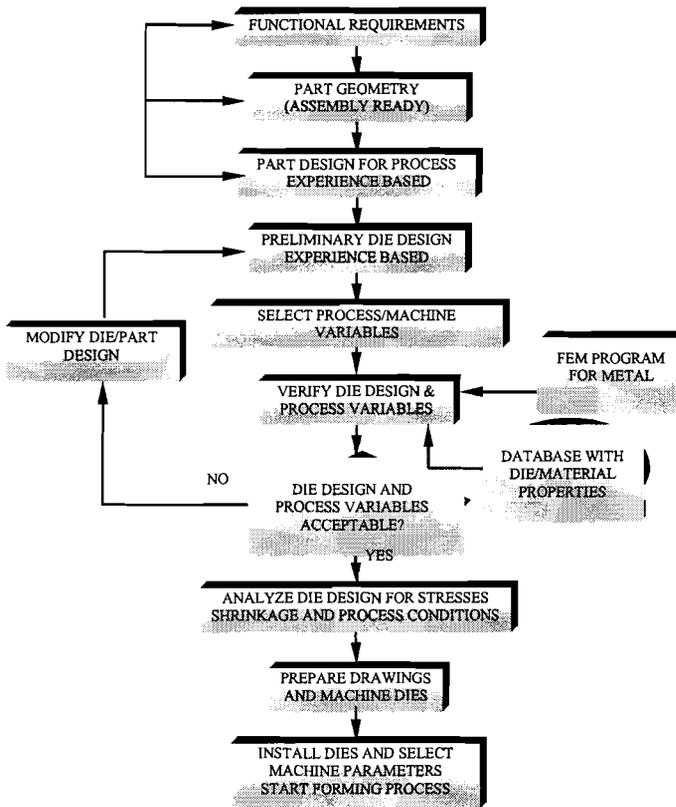
**Figure 3. Product & Process Design for Net Shape Manufacturing**
