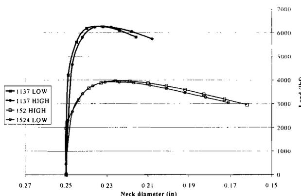
5. NECK DIAMETER-LOAD CURVE FOR TENSILE TESTS WITH NOTCHED SPECIMENS OF SAE 1137 HOT ROLLED AND SAE 1524 SPHEROIDIZED ANNEALED.
