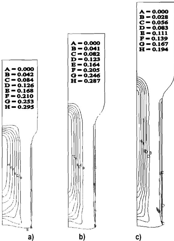
10. DISTRIBUTION OF THE DAMAGE VALUE DURING SEVERAL REDUCTIONS IN AREA: (A) 30%, (B) 45% AND (C) 55% (B = 0.150" AND R = 0.200").
