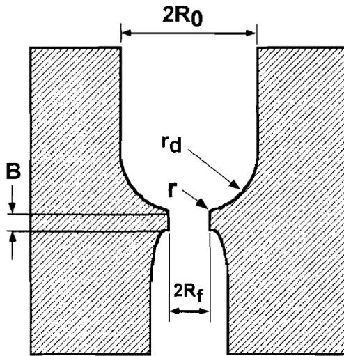
7. SCHEMATIC REPRESENTATION OF THE PARAMETERS TO BE INVESTIGATED DURING THE FORWARD EXTRUSION WITH SPHERICAL DIE.
