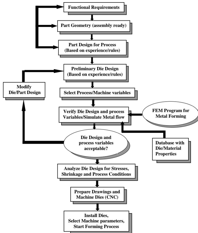
**Figure 1: A flow chart illustrating forging process design (2).**
