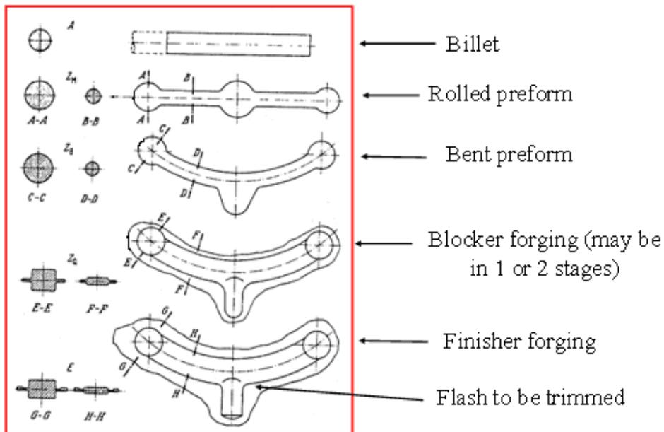
**Figure 2: Illustration of the hot forging sequence for upper control arms using an example part (5).**
