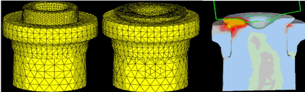
**Figure 8: FE simulation of orbital forming (FE model and stress distribution) (9).**
