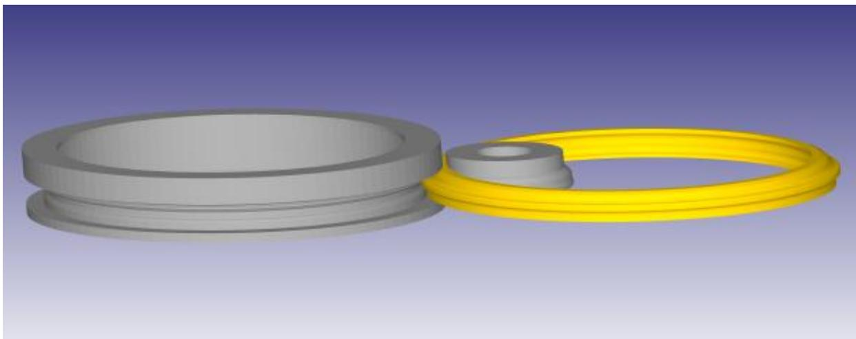
**Figure 9: An aerospace component is shown at the end of a ring rolling process**
