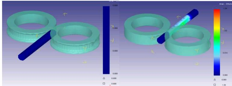
**Figure 3: Simulation of the reducer rolling process.**
