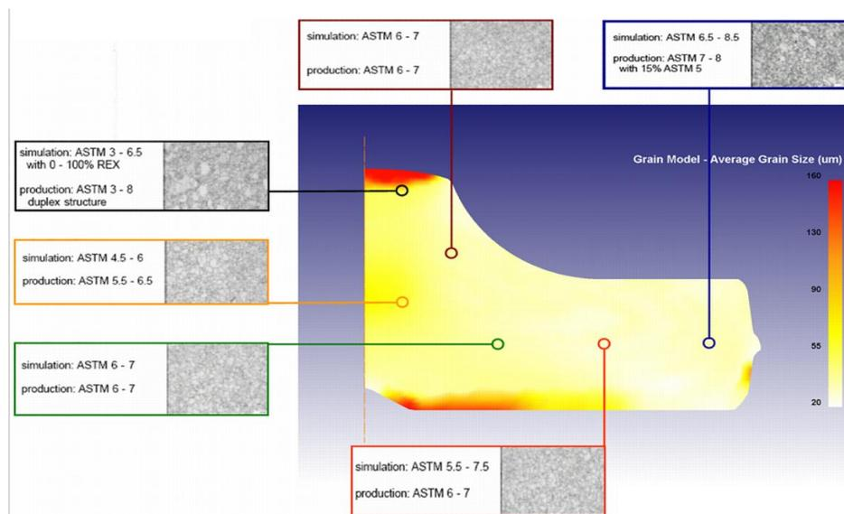
Figure 10: The correlation between the simulation and production grain size [12]
