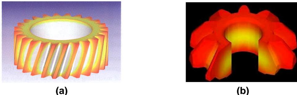
Figure 7: Heat treatment simulations of gears (11).
