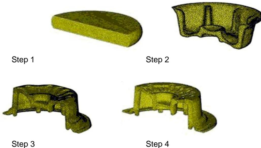
**Figure 11: Forging sequence of the aircraft wheel (part geometry courtesy of Weber Metals Inc.) (5).**
