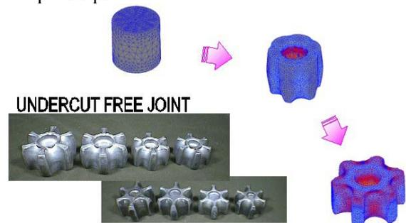
Fig 20: Cold forging of the inner race of a CVJ [14].
