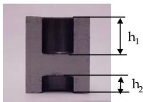
Fig. 3: Specimen showing the cup heights after the double-cup extrusion test.
