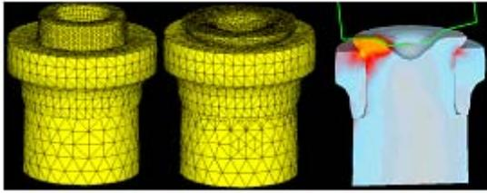
Fig 8: FE simulation of orbital forming (FE model and Stress distribution)
