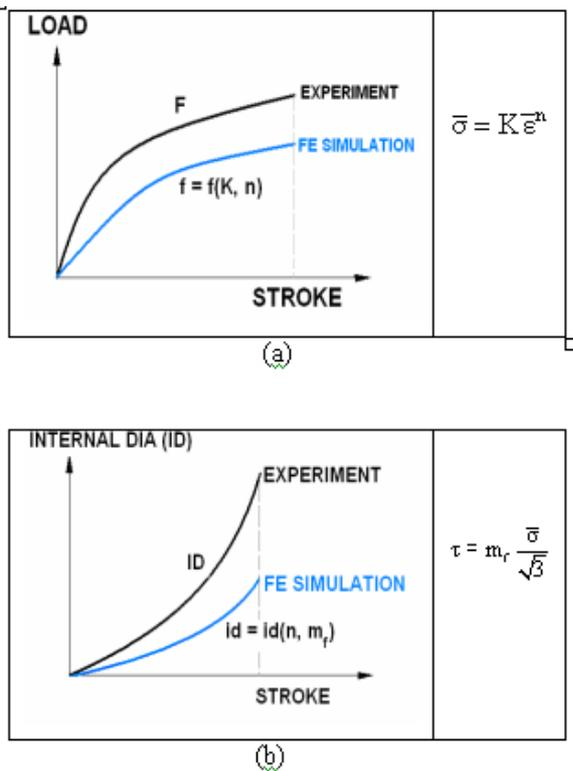
Fig. 6: Methodology for simultaneous determination of friction and flow stress by inverse analysis.
