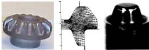
Fig 16: Bevel gear, FE model and the punch used to forge the gear [13].
