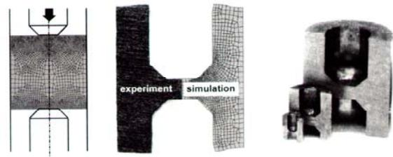
Fig 9: Double cup extrusion test for determination of friction conditions in microforming [10].
