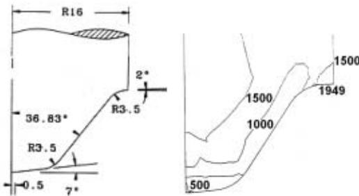
Fig 18: Stress contours in the punch after geometric modifications.
