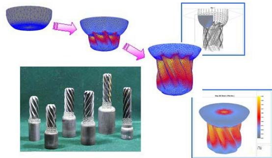
Fig 19: Development of steering pinion with the aid of FE simulation [14].
