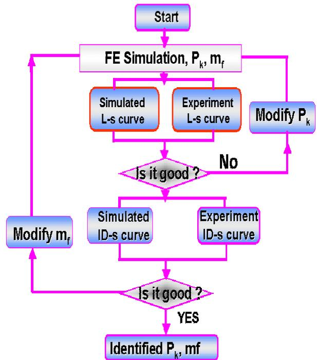
Fig. 7: Flow chart of inverse analysis procedure.
