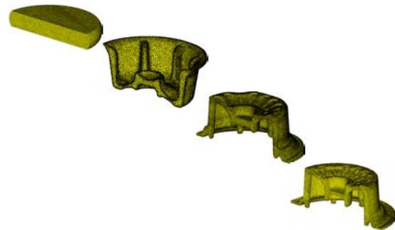
Fig 15: Aircraft landing gear wheel (Wheel diameter = 560 mm, Height = 216 mm; No of elements = 60,000), by ERC/NSM [12].
