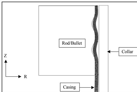
Fig. 13: FE model for the rod pullout test.
