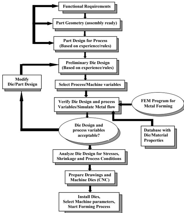
Fig. 1: A flow chart illustrating forging process design [2].
