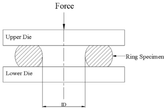
Fig. 5: Schematic diagram of the ring compression test.
