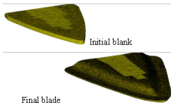
Fig 9: Microforming of surgical blades (Blank thickness = 0.1 mm; Final blade thickness = 0.01 mm) [9].
