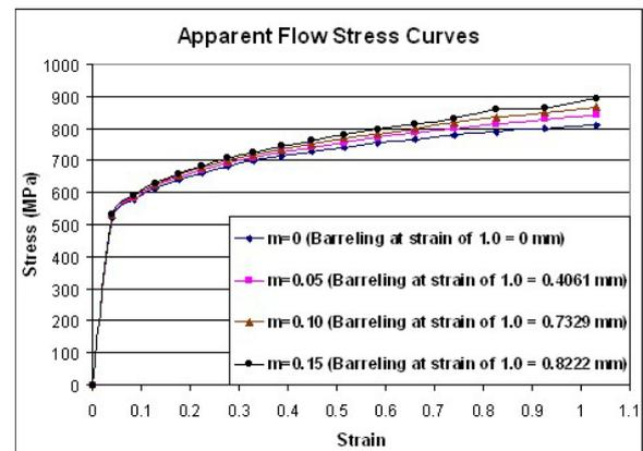
c) Flow stress curves obtained from FE simulations
