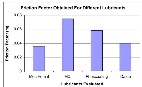
Fig. 4: Ranking of the lubricants based on the friction factors obtained.
