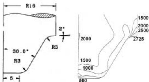
Fig 17: Stress contours in the punch before geometric modifications.
