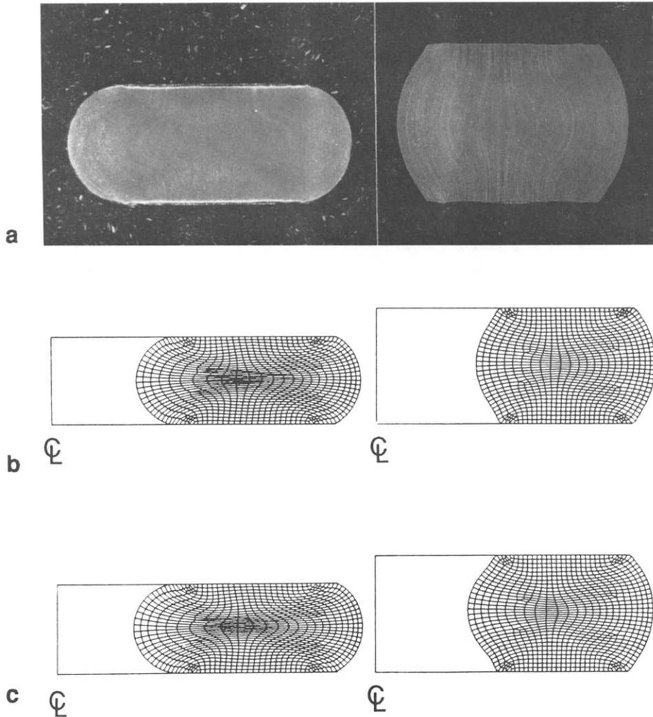
Fig. 5. Comparison of ring cross sections at 26% and 45% reductions for Ti-6Al-4V ring compression tests: (a) experimental observations [2]; (b) FEM simulations with flow stress corrected by temperature compensation scheme, eqn. (1), with  $F(t)$  from eqn. (2); and (c) FEM simulations with the isothermal flow stress data after correction for deformation heating. (Ram speed=5.1 mm/s (0.2 in/s); friction shear factor  $m=0.18$ .)
