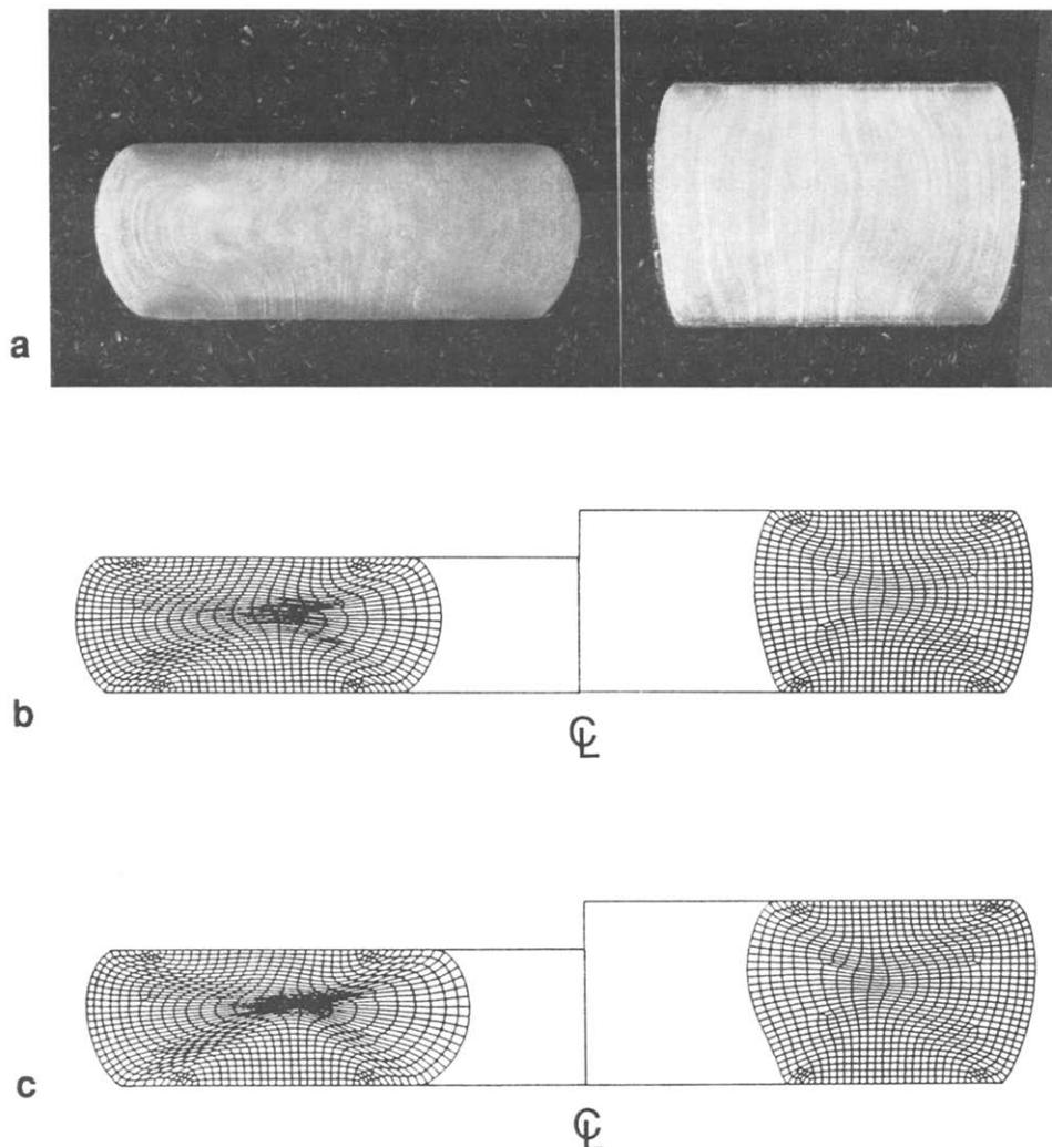
Fig. 8. Comparison of ring cross sections at 30% and 49% reductions for Ti-6Al-4V ring compression tests: (a) experimental observations [2]; (b) FEM simulations with flow stress corrected by temperature compensation scheme, eqn. (1), with  $F(t)$  from eqn. (2); and (c) FEM simulations with the isothermal flow stress data after correction for deformation heating. (Ram speed = 56 mm/s (2.2 in/s); friction shear factor  $m = 0.16$ .)
