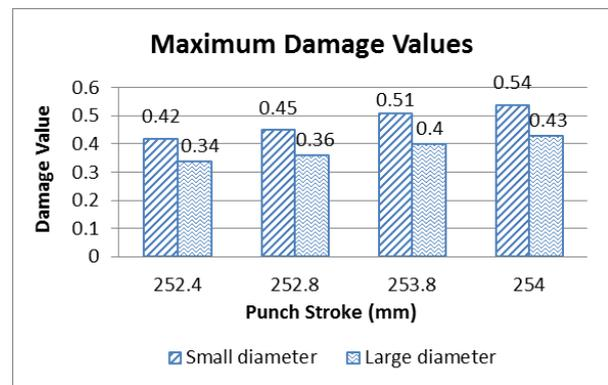
Figure 3: Maximum damage values, estimated for coining preforms with different head diameters
