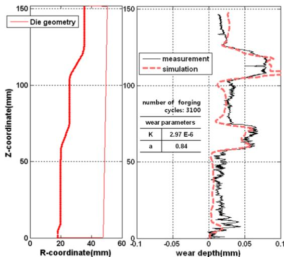
Figure 1: Predicted wear from FE simulation versus CMM measured wear compensating for the plastic deformation for Extrusion Insert (3100 Cycles)
