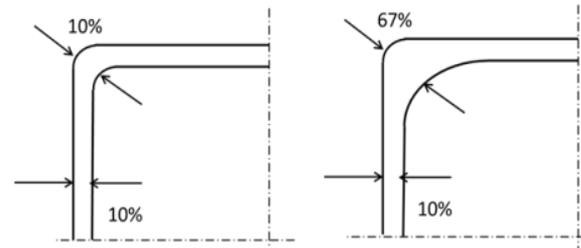
Figure 6: Different clearances around the corner radius of a rectangular punch used in [8]
