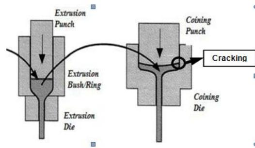
Figure 2: Extrusion of a preform (left) and coining of the valve head (right) in forging engine valves
