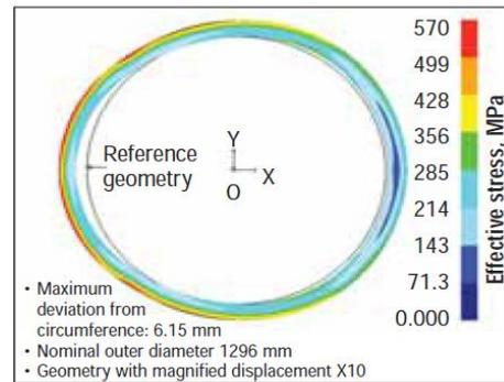
Figure 4: Geometrical distortion and residual stresses after FE simulation of heat treatment
