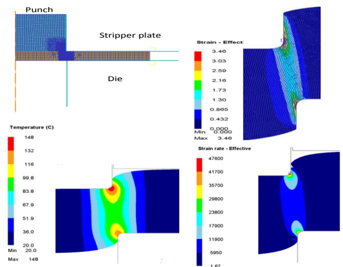
Figure 5: (from top left clockwise) FE model setup; strain distribution; strain rate distribution; temperature distribution in the sheet during blanking of 0.2mm thick C51100 sheet
