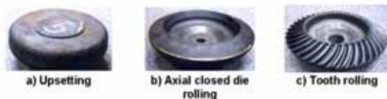
Figure 11: Axial closed die rolling sequence for a bevel gear [15].
