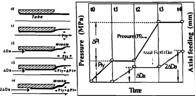
Figure 13: Adaptive simulation procedure.  $P_{iy}$ : yielding pressure;  $\Delta P_i$ : pressure increment;  $\Delta D_a$ : axial feed increment [14].
