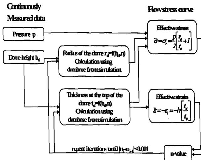
Figure 19: Determination of flow stress curve for sheet metals [23]
