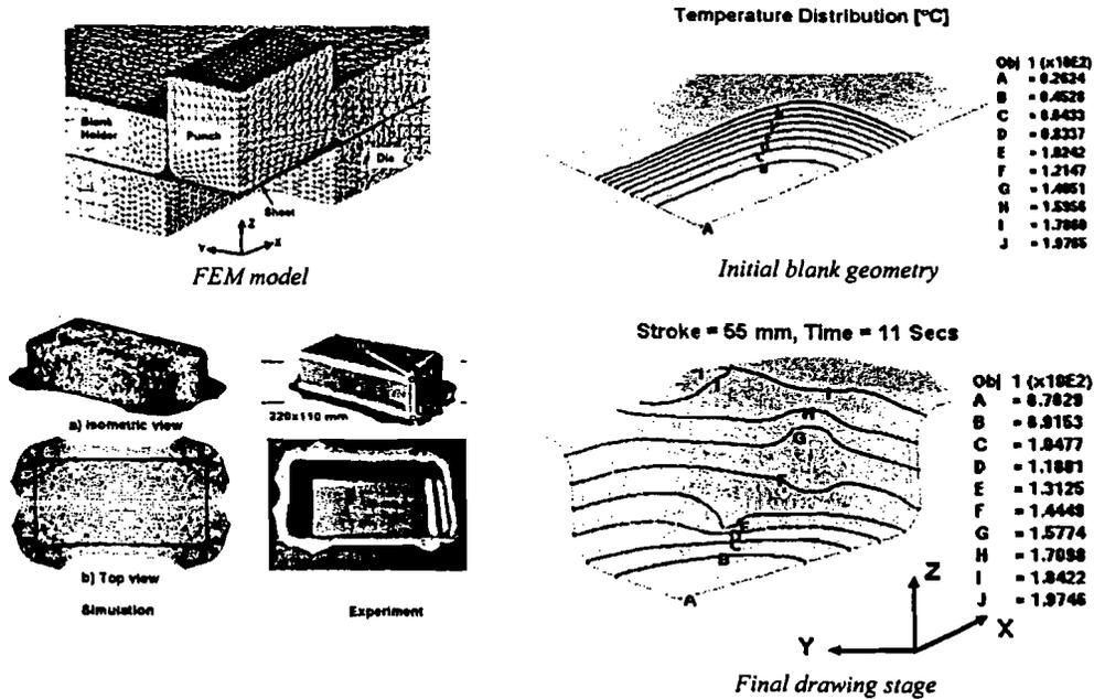
Figure 8: Rectangular pan warm sheet forming process in DEFORM 3D (Experiments were conducted by Droder [12])
