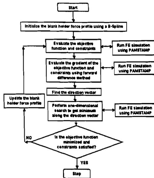
Figure 9: Flowchart of the optimization algorithm for determining optimum variable BF profiles[13]
