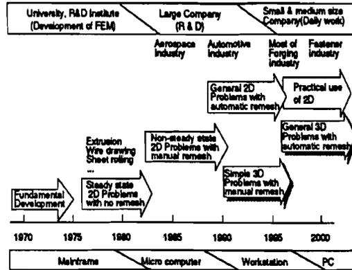
Figure 1: History of practical use of FE simulation in forging [1]
