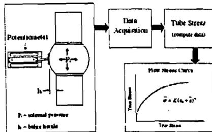
Figure 20: Bulge test for flow stress measurement of tubular materials [23]
