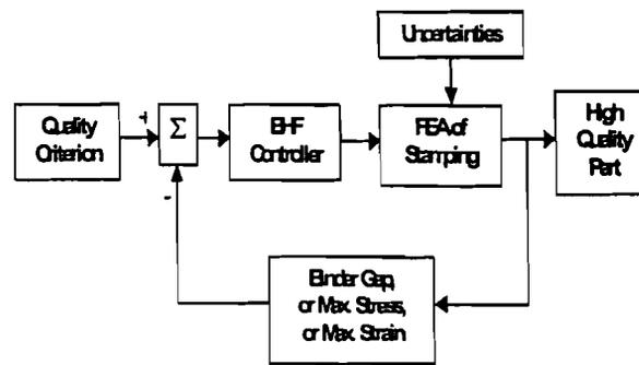
Figure 10: Feedback algorithm for calculating optimal time and location variable BF profiles using commercial FEM software - adaptive simulation[13].
