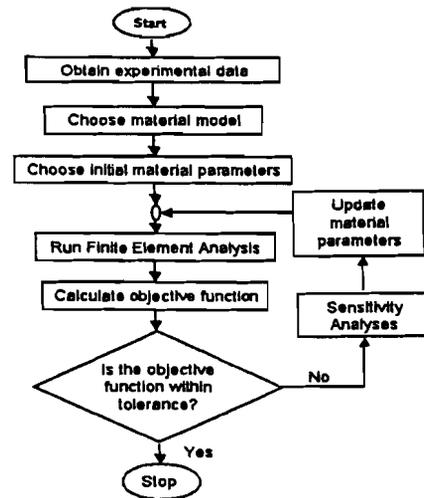
Figure 21: Flowchart for inverse analysis to identify the material parameters [30].
