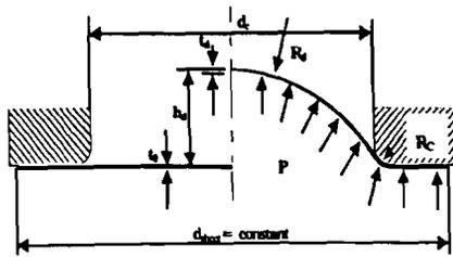
Figure 18: Geometry of the bulge test (sheet)
