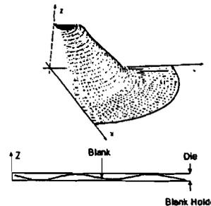
Figure.11: Definition of flange wrinkle constraint function[13]
