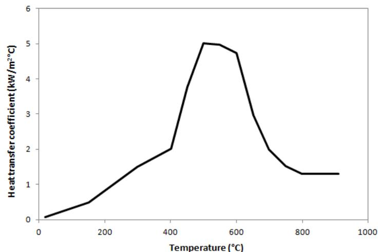
Figure 5 – Heat transfer coefficient between AISI 4140 and still oil (Hardin and Beckermann, 2005).
