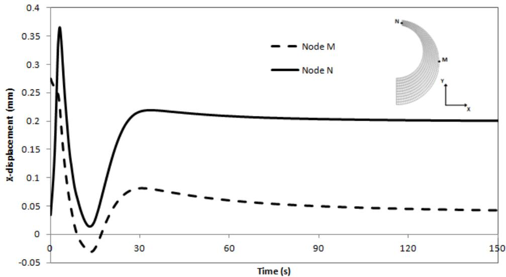
Figure 8 – Simulated displacements in the x direction for Nodes *N* and *M* of the C-ring, during the oil quenching process.
