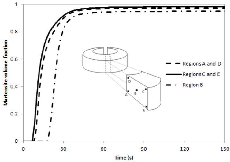
Figure 12 – Simulated evolution of the martensite volume fraction at several points in the transversal cross-section of the C-ring during oil quenching.
