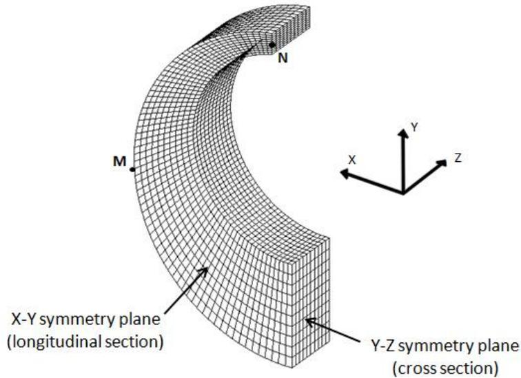
Figure 6 – Meshed  $\frac{1}{4}$  symmetric geometry, used for the simulation. Nodes *M* and *N* were used for outside diameter and gap opening evaluation, respectively.
