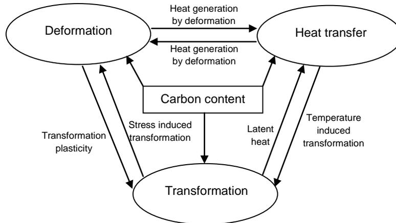
Figure 4 - Coupled phenomena considered during the quenching simulations.
