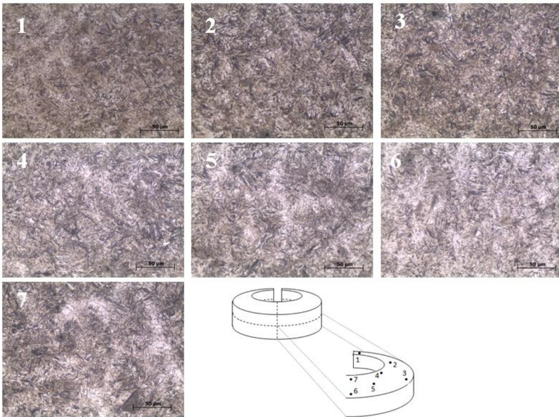
Figure 10 – Micrographs from various points in the longitudinal cross-section of a C-ring, indicating the presence of martensite in all locations (optical microscopy).
