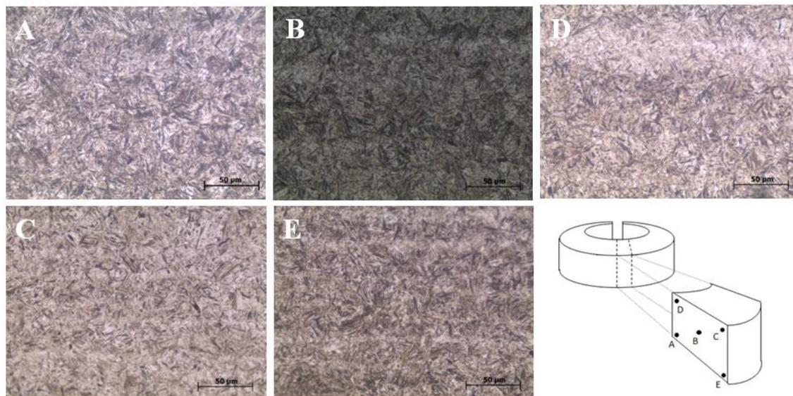
Figure 9 – Micrographs from various points in the transversal cross-section of a C-ring, indicating the presence of martensite in all locations (optical microscopy).
