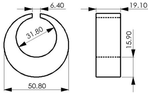
Figure 1 – C-ring geometry (all dimensions in mm).
