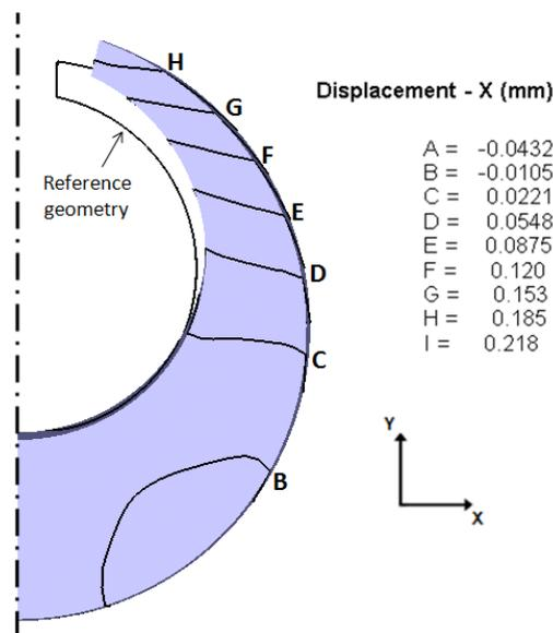
Figure 7 – Simulated displacement in the x direction of the points in the longitudinal cross-section of the C-ring (displaced geometry magnified 20x).
