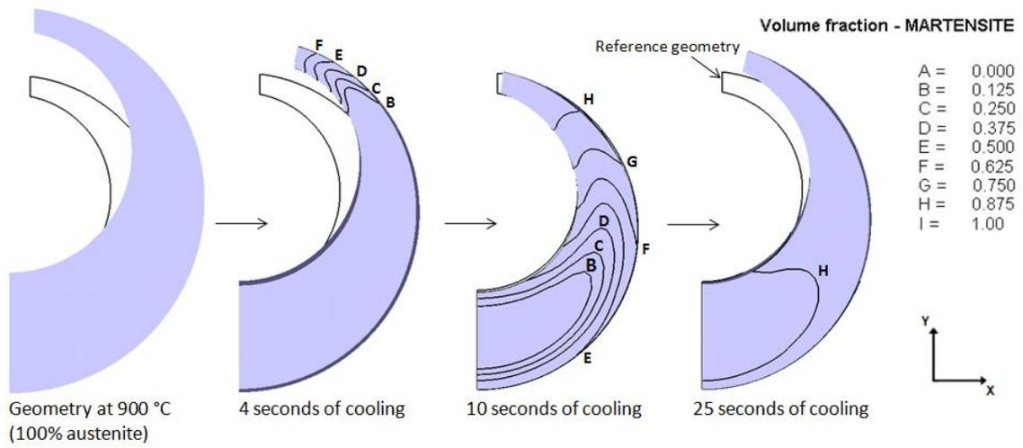
Figure 11 – Martensite formation (displaced geometry magnified 20x) on the C-ring during the cooling simulation.
