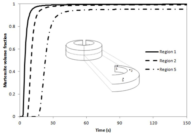
Figure 13 – Simulated evolution of the martensite volume fraction at several points in the longitudinal cross-section of the C-ring during oil quenching.
