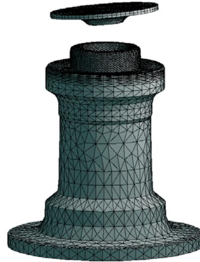
Figure 8: 3D Finite element model for orbital forming simulation.
