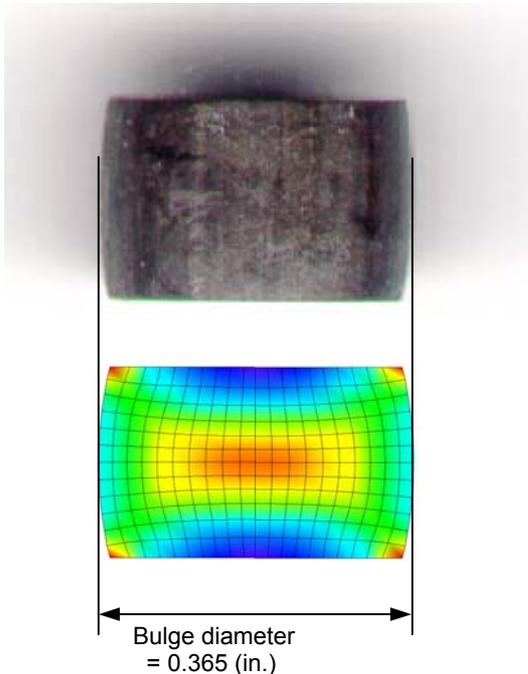
Figure 4: Comparison of measured (top) and computed (bottom) bulge diameters at the end of stroke with  $\bar{\sigma} = 113\bar{\epsilon}^{0.138}$  (Mpa) and  $m_f = 0.15$ .
