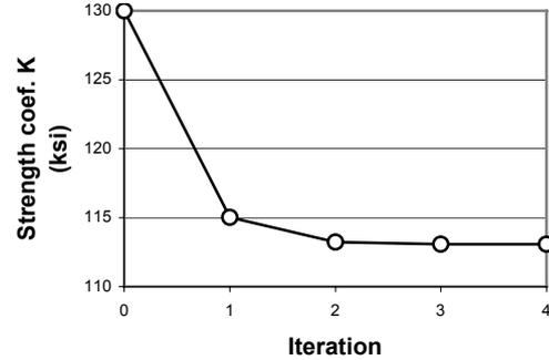
Figure 5: Convergence of material strength coefficient, K.
