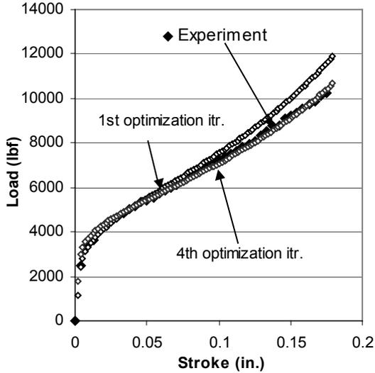
Figure 3: Comparison of computed and experimental load stroke curves.
