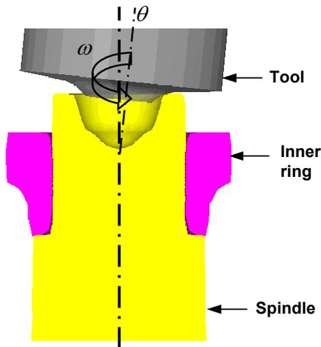
Figure 7: Principle of orbital forming of wheel spindle bearing.
