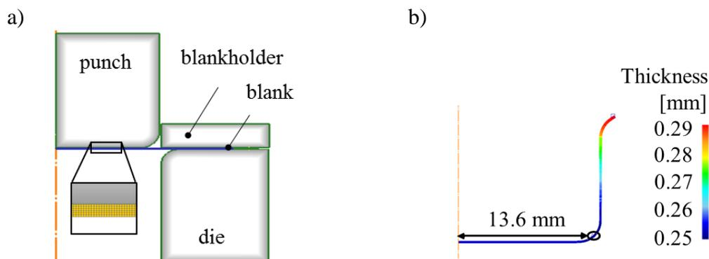
**Figure 3.** Illustration of the a) initial numerical model, and b) location of maximum thinning at the end of the first drawing stage calculated with optimized process parameters.
