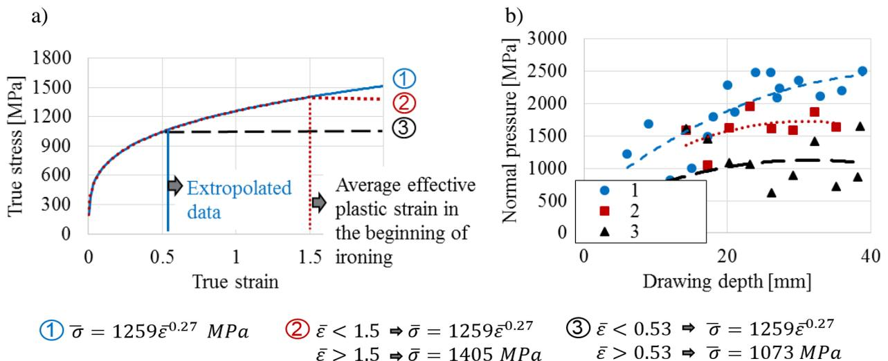
**Figure 8.** a) Various stress-strain curves used for numerical analysis of ironing stage and b) corresponding contact pressure as a function of drawing depth (Numbers 1, 2 and 3 correspond to various flow stress curve cases).
