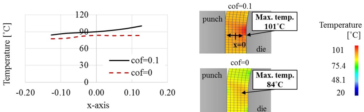
**Figure 6.** Temperature distribution along the cross section of blank for  $\text{cof}=0$  and  $\text{cof}=0.1$ .
