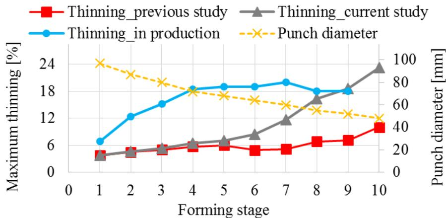
**Figure 2.** Maximum thinning and punch diameter with respect to forming stages for existing part, Part A.
