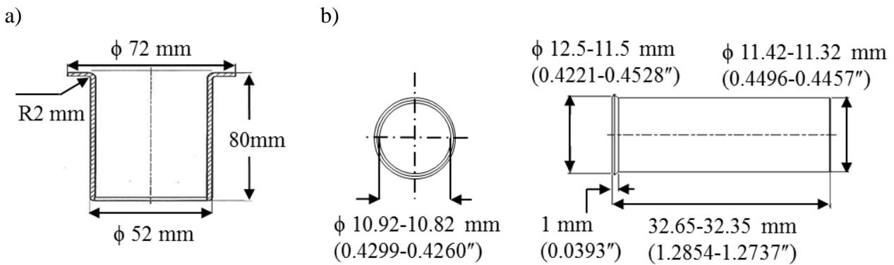
**Figure 1.** Geometry of a) example existing part (Part A, AISI 1008), and b) current part (Part B, AISI 305).
