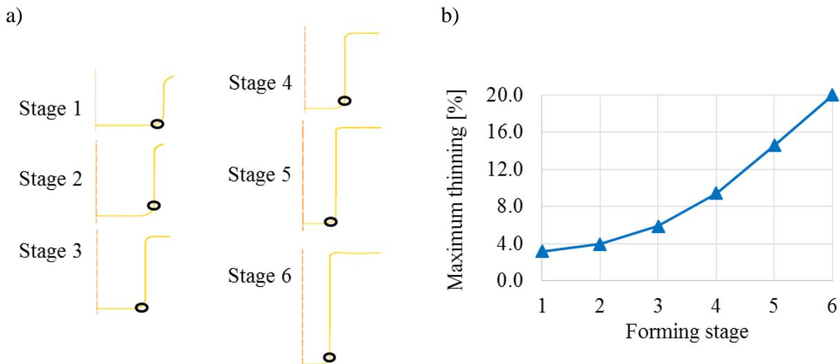
**Figure 4.** a) Deformed part geometry after each forming stage with the detail of maximum thinning region, illustrated with an ellipse and b) maximum wall thinning as a function of forming stage.
