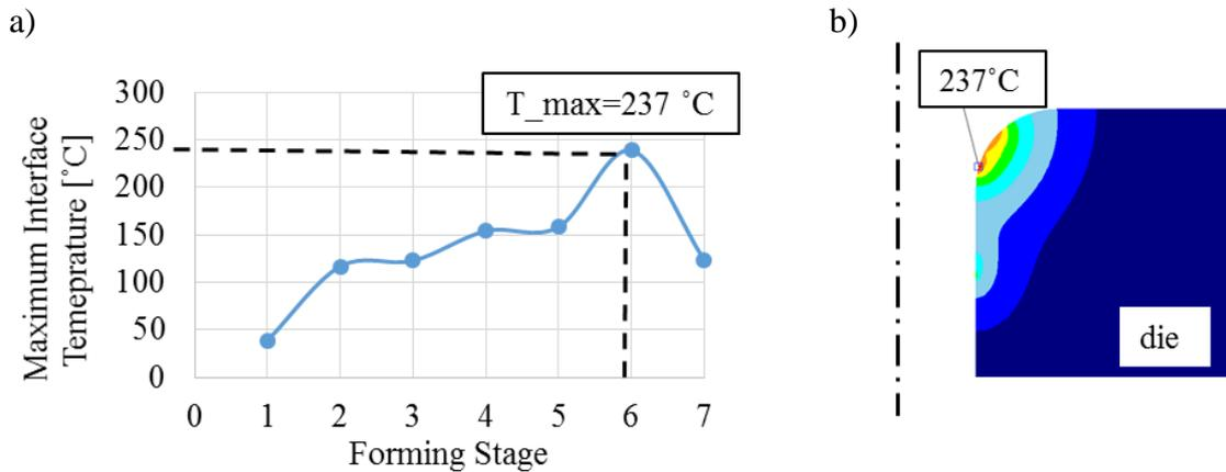
**Figure 7.** Illustration of a) calculated maximum contact die temperature with respect to drawing stages and b) temperature distribution in lower die at Stage 6.
