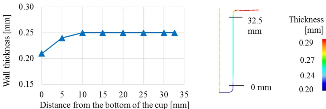
**Figure 5.** Wall thickness distribution of the ironed part with respect to distance from the bottom of the cup.
