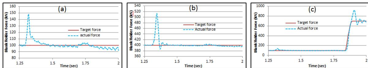
Figure 2. Three different BHF used in the tests. (a) constant 100 kN, (b) constant 400 kN, (c) variable 100 to 700 kN. The solid lines show the target force and the dashed lines indicate the actual force applied by the cushion.
