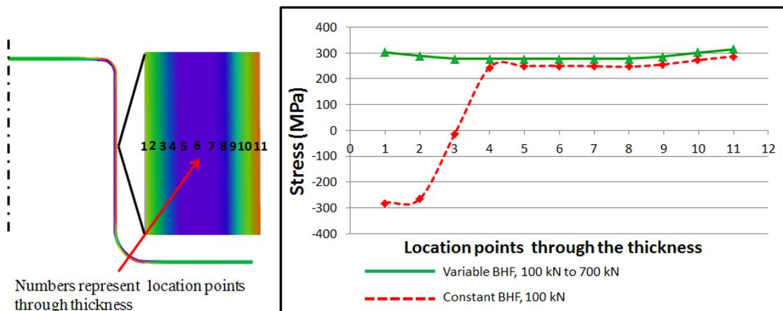
Figure 4. Stress distribution along the sheet thickness at wall area for two different BHF values
