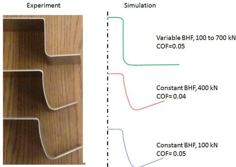
Figure 3. Experimental results and simulation predictions of springback for 3 different BHF values
