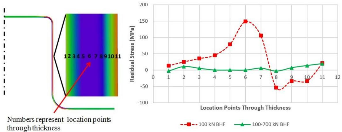
Figure 5. Residual stress distribution along the sheet thickness
