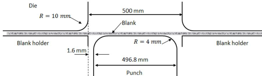
Figure 1. A schematic of tools and dimensions for the U-draw bending.
