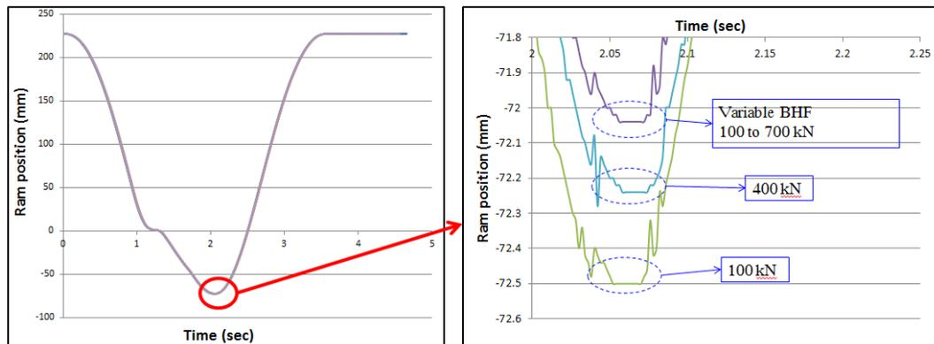
Figure 7. Measured die displacement versus time for three different BHF's.
