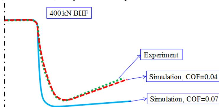
Figure 6. Effect of COF on springback prediction
