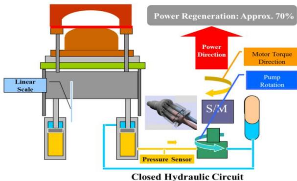
Figure 13: Servo-hydraulic cushion with power regeneration [courtesy Aida]
