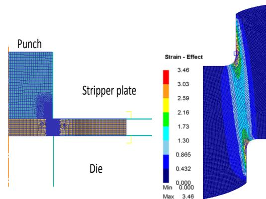
Figure 6: (left) FE model setup;(right) strain distribution in the sheet during blanking of 0.2 mm thick C51100 sheet
