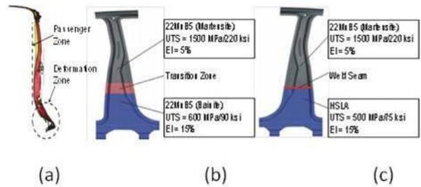
Figure 11: (a) Side view of a B-pillar after crash, (b) Tailored properties or (c) TWBs may improve elongation in the deformation zone[9]
