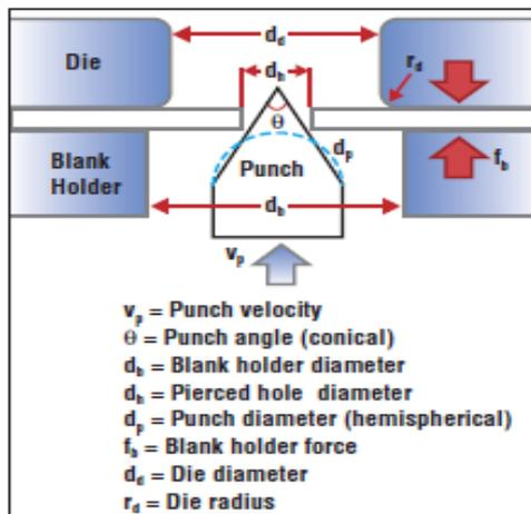
Figure 9: Hole expansion test schematic
