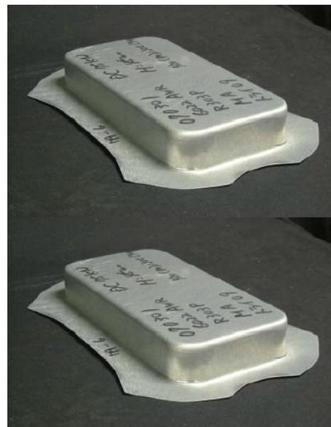
Figure 15: panel formed at (a) 41 mm/s and (b) 103 mm/s [12]
