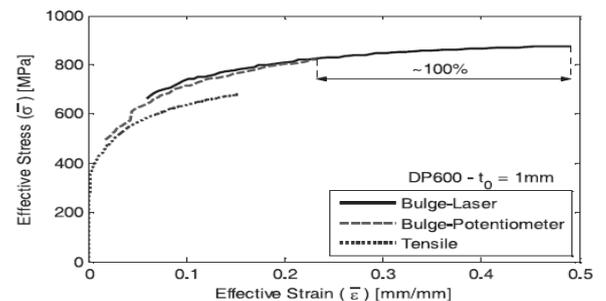
Figure 2: Comparison of flow curves determined to determine flow stress curves for larger strains. [1] by VPB and tensile test [3]
