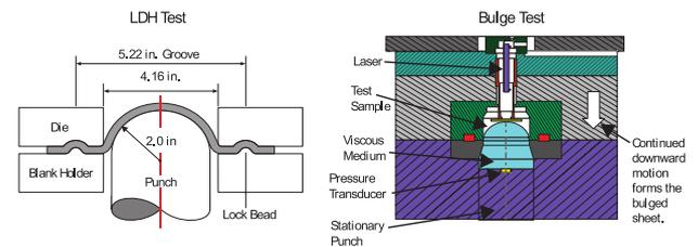
Figure 1: Schematic of the biaxial LDH and VPB tests
