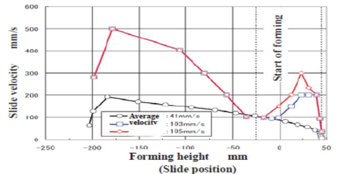
Figure 14: different slide motions used to form panels [12]
