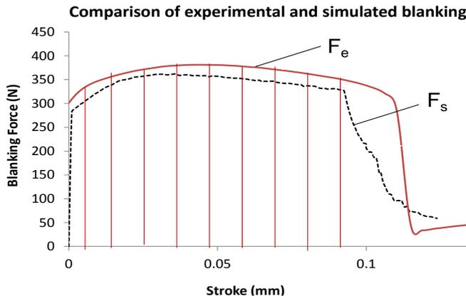
Figure 7: Comparison of experimentally obtained and simulated blanking force at small intervals of stroke to obtain high strain and strain rate flow stress
