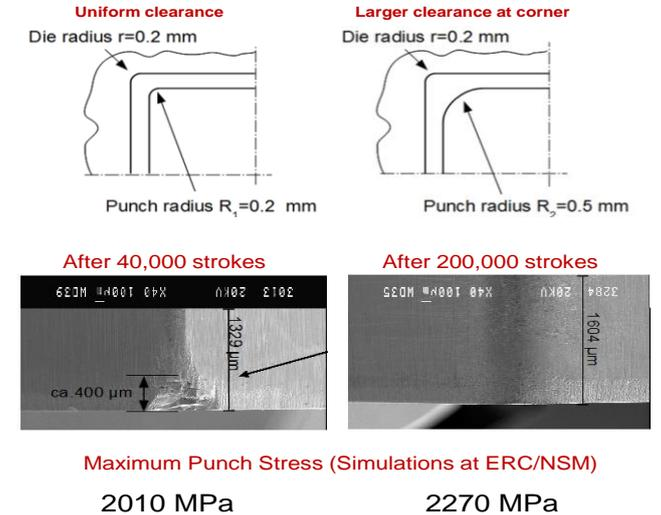
Figure 8: Effect of punch-die clearance on tool wear in experiments and tool stress in simulations
