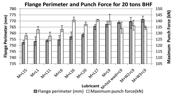
Figure 5: Flange perimeter and punch force recorded for 20 tons BHF (one lubricant condition failed at 20 tons) [5]
