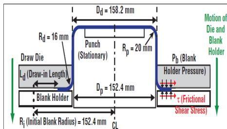
Figure 4: Cup drawing test schematic [4]
