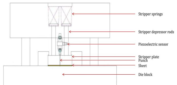
Figure 1: Experimental setup for punch force measurements (schematic)
