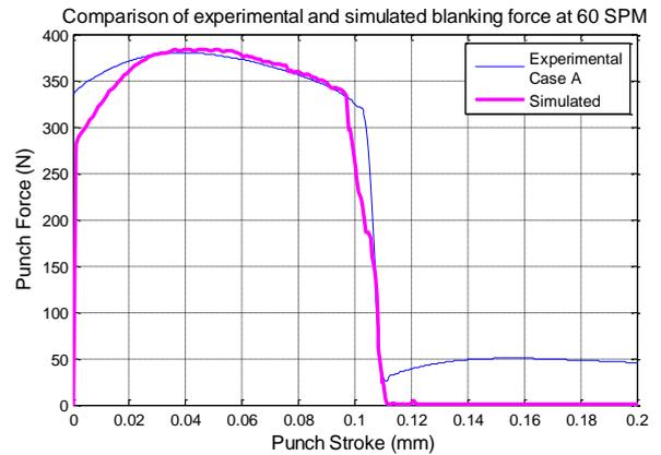
Figure 7: Comparison of experimental and simulated blanking load [The initial elastic portion of the experimental curve was not included in the comparison since it could not be replicated in the simulation]
