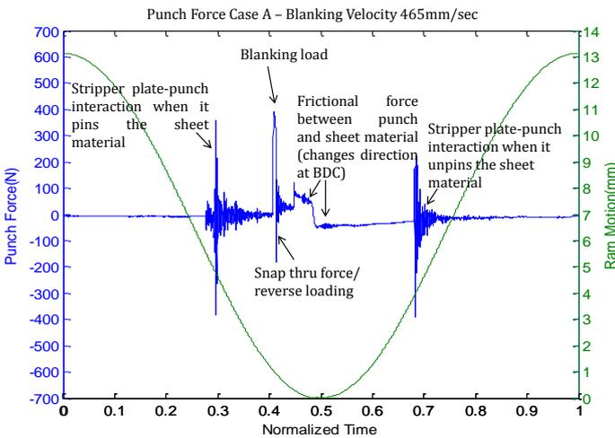
Figure 2: Forces acting on the punch during blanking
