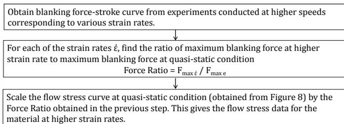
Figure 10: Flow chart to develop flow stress curve using blanking tests for higher strain rate
