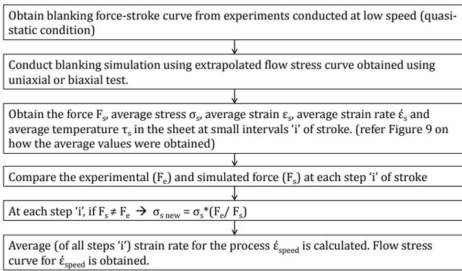
Figure 8: Flow chart to develop flow stress curve using blanking tests for low strain rate
