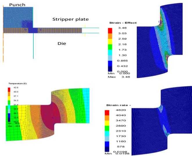
Figure 6: (From top left clockwise) FE model setup; strain distribution; temperature distribution in the sheet (at 0.1mm punch stroke / sheet thickness = 0.2mm)
