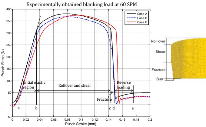
Figure 5: (left) Blanking load curve at 60 SPM; (right) blanked edge profile
