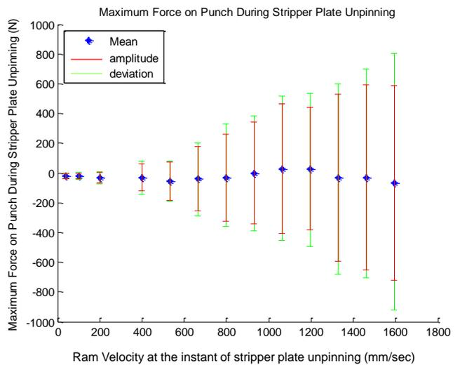
Figure 4: Influence of velocity on vibrations during stripper unpinning
