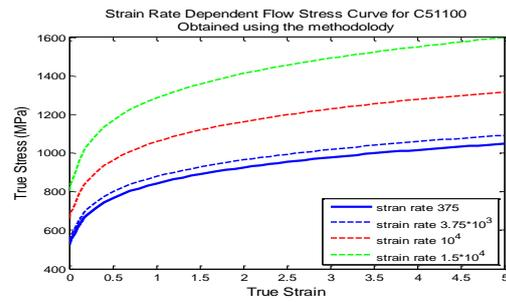
Figure 11: Flow stress for C51100 obtained using the methodology
