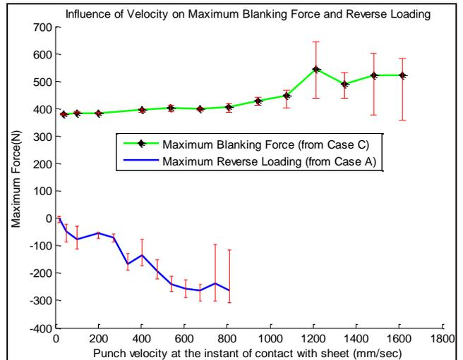
Figure 3: Influence of velocity on maximum blanking force and maximum reverse load
