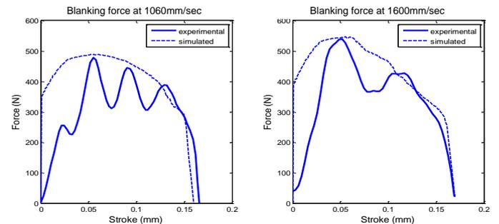
Figure 12: Comparison of blanking force obtained from simulation and experiments
