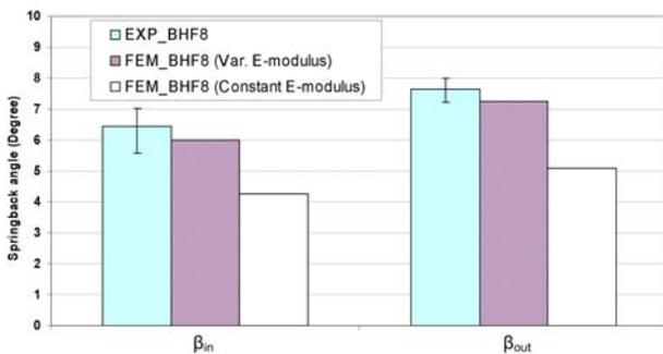
**Figure 8.** Comparison of springback angle in the flange areas between FEM predictions and experiments.
