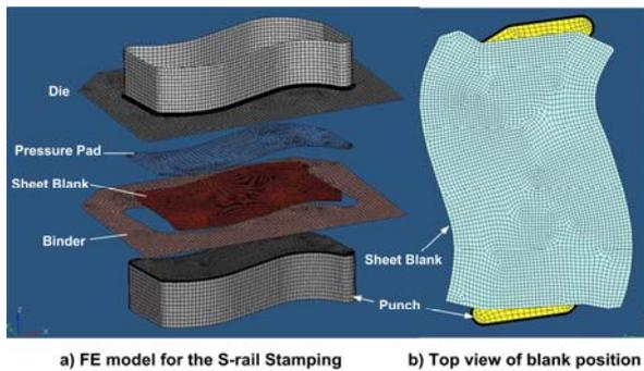
**Figure 12:** S-Rail stamping simulation model and the configuration of the initial position of blank.
