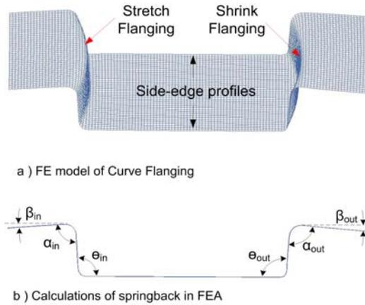
**Figure 7.** Locations of the measurements for various angles after springback.
