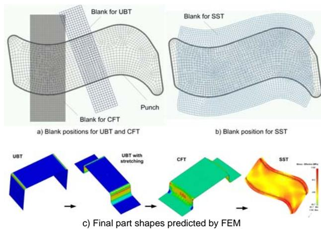
**Figure 1.** Schematic of various forming tests with S-shaped tooling and the final shape predicted by FEM.
