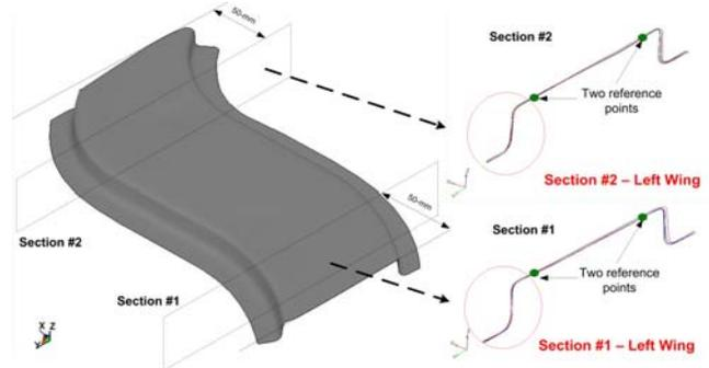
**Figure 13:** Two selected sections for springback comparison.
