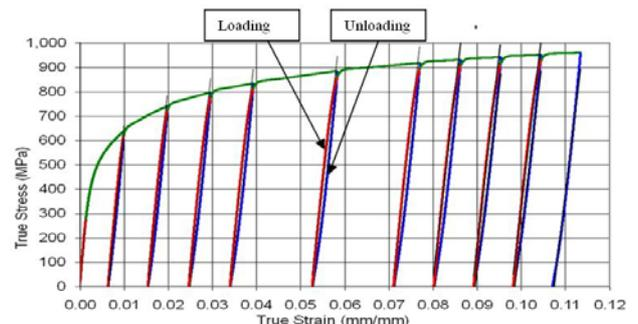
**Figure 3.** True stress-strain curves in the loading and unloading tensile test for DP 780 material.
