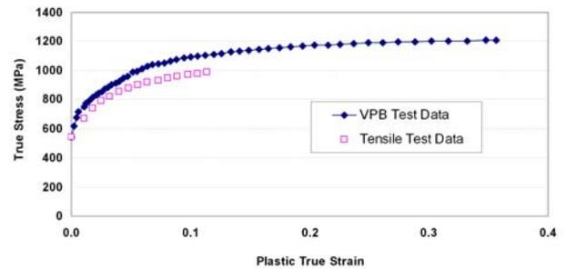
**Figure 2.** True stress-strain data obtained from the VPB test and tensile test for DP 780.
