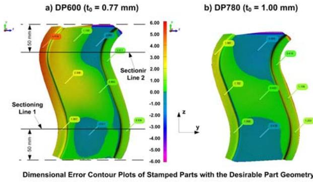
**Figure 11.** Springback measurements for DP 600 and DP 780 stampings with the designed part geometry (all dimensions shown are in millimeters).
