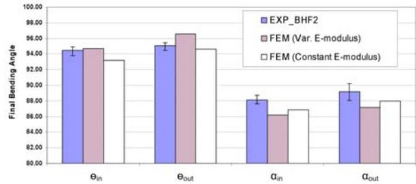
**Figure 9.** Comparison of the final bending angles of curved flanging between FEM predictions and experiments at a BHF of 8 tons.
