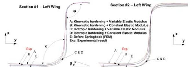
**Figure 14:** Comparison of FEM predictions and experiment.
