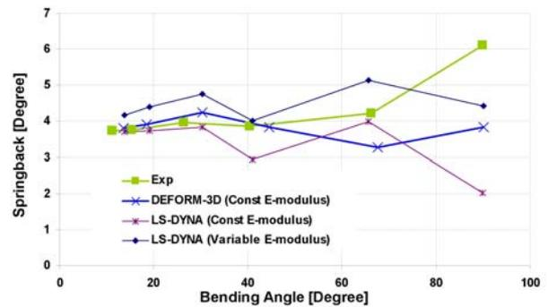
**Figure 5.** Comparison of springback between FEM predictions and experiments of DP 780 in U-shaped free bending.
