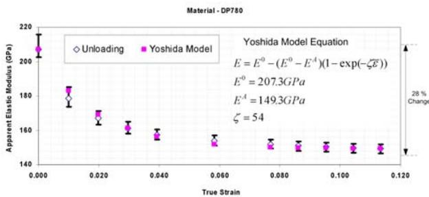
**Figure 4.** Yoshida model vs. experimental data for variable elastic modulus of DP 780.
