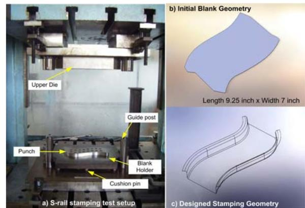
**Figure 10.** S-Rail tooling and the geometries of the initial blank and final stamping.
