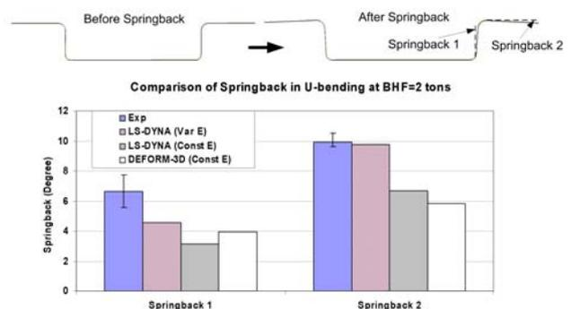
**Figure 6.** Comparison of springback in U-shaped stretch bending of DP 780 at a BHF of 2 tons.
